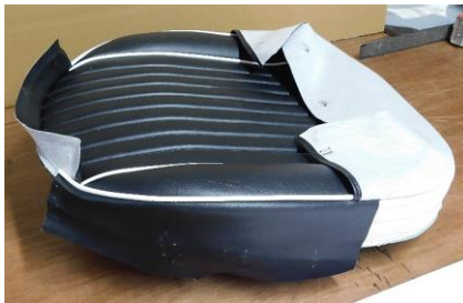
B28) Holding the frame in place, turn the assembly over, fold the rear side skirts over the sides of the assembly – as shown above right.
