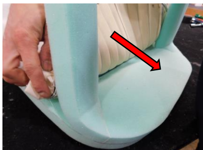
B20) Pull the seat cover forward so that the flutes lay over the front roll.
