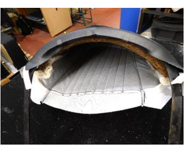
22) Continue to manipulate the cover by firmly smoothing your hands in a generally downwards direction, working out any creases and ensure the outer piping sits on the frame edge. Once in a satisfactory position, clip the back of the cover over the lower frame edge. Three clips will do at this stage.
