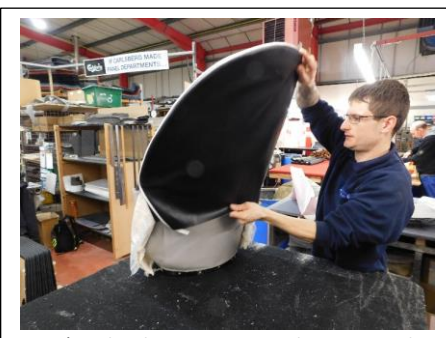
20) Take the correct Squab Cover and begin to slide it down over the frame/padding to approximately half way.
