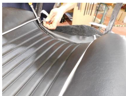
37) Trim off any excess & fold the trimmed front flap under the rear flap to give a neat finish.
