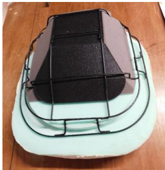
B27) Place the wire frame centrally over the base foam.
