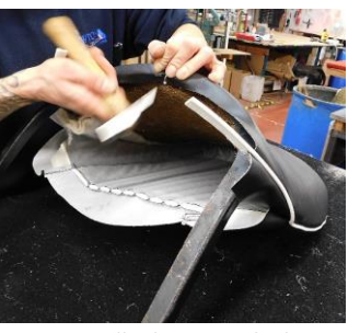
22) Continue to manipulate the cover by firmly smoothing your hands in a generally downwards direction, working out any creases and ensure the outer piping sits on the frame edge. Once in a satisfactory position, clip the back of the cover over the lower frame edge. Three clips will do at this stage.
