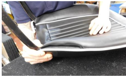
32) Tuck the side edges at the bottom of the horseshoe under to make a neat finish. Smooth them flat with your hand.
