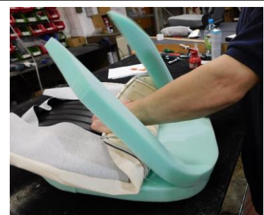
B19) Carefully position the Top Roll foam in place over the front of the Base foam with the front of the Seat Cover lifted up. Out of the way. Make sure the back edge of the roll aligns with the line marked across the front of the base pad & that all outside edges line up. When satisfied that all is well, press firmly together.
