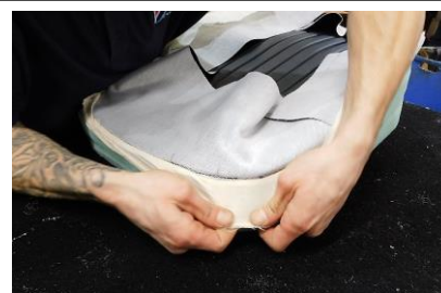
B24) Carefully pull the calico flap out and over the edge of the foam assembly, pulling out creases as you go.
