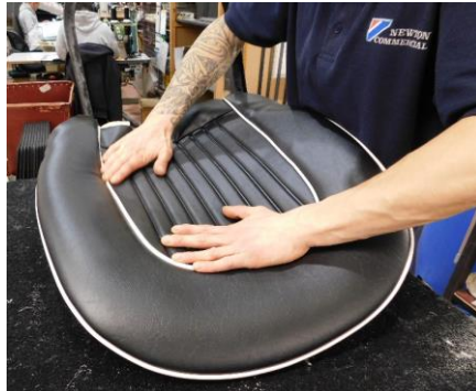
31) Lay the seat on its back. It is now time to push the two glued surfaces together. Starting at the top, push the centre fluted area down onto the padding, ensure that the flutes are vertical and that there are no creases in the horseshoe surround. The cover should be a tight enough fit to avoid any creasing. Push down firmly over the whole fluted area.
