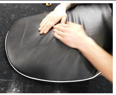
21) At the wide point of the frame, firmly grasp the seat cover where the front horseshoe joins the outer piping on both sides. (These are the weak points of the cover which need protecting so that they do not tear when pulling the cover down further) Now pull the cover fully downwards over the wide point, so that it is roughly in the correct position. Using the flat of the hand, gradually work the cover in a downwards
