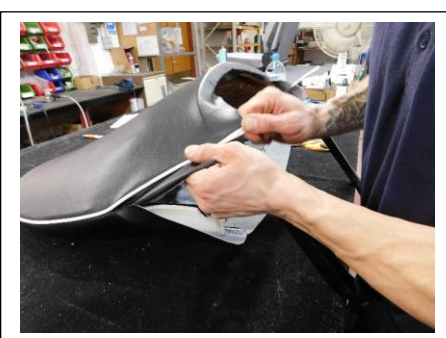
25) Pull the piping down over the frame. This should remove any creases at the side. At the same time firmly smooth the piping downwards from the top of the seat whilst maintaining a good tension all around the cover.
