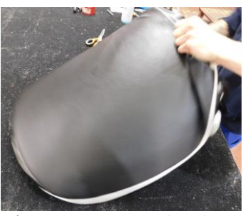
22) Continue to manipulate the cover by firmly smoothing your hands in a generally downwards direction, working out any creases and ensure the outer piping sits on the frame edge. Once in a satisfactory position, clip the back of the cover over the lower frame edge. Three clips will do at this stage.
