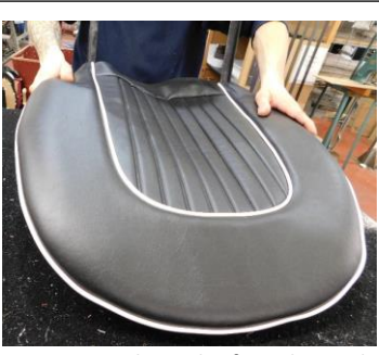
21) At the wide point of the frame, firmly grasp the seat cover where the front horseshoe joins the outer piping on both sides. (These are the weak points of the cover which need protecting so that they do not tear when pulling the cover down further) Now pull the cover fully downwards over the wide point, so that it is roughly in the correct position. Using the flat of the hand, gradually work the cover in a downwards
