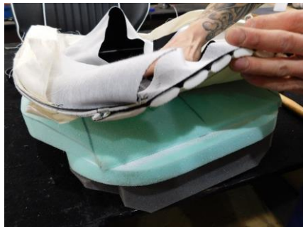
B13) Line up the centre lines & the piped edges with the outside lines, then press down firmly so that cover is fixed to the base foam within the marked lines.
