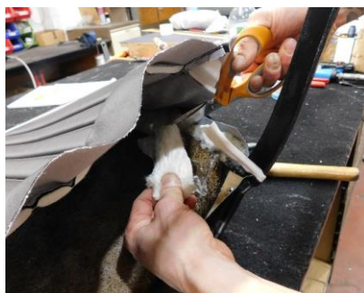
28) Remove the wadding from this area, using scissors to trim it away, just leaving the 'horsehair'. Repeat for the other side.
