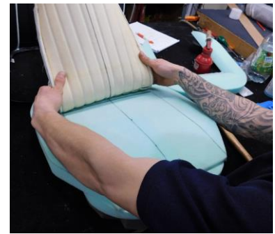
B12) Starting at the front of the glued areas, place the cover carefully on the foam
