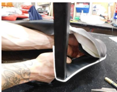
27) Now we look at the inner bottom flaps on the piping. Pulling the flap inwards, you can see that it needs to lie flat onto the padding.
