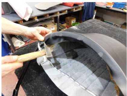
26) Having pulled the piping over the edge of the frame, the cover next to the piping can be clipped to the base frame – Repeat for the other side.
