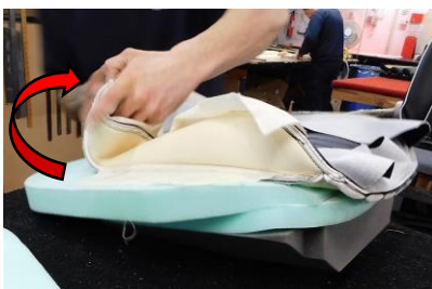
B18) Lift the base cover away from the side & front roll areas, exposing the base foam. Spray glue across the front of the base foam
