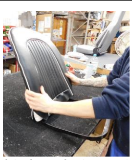
21) At the wide point of the frame, firmly grasp the seat cover where the front horseshoe joins the outer piping on both sides. (These are the weak points of the cover which need protecting so that they do not tear when pulling the cover down further) Now pull the cover fully downwards over the wide point, so that it is roughly in the correct position. Using the flat of the hand, gradually work the cover in a downwards
