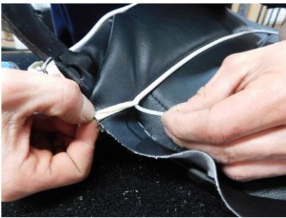
34) Remove the piping core (as before) from the piping tails at the front.
