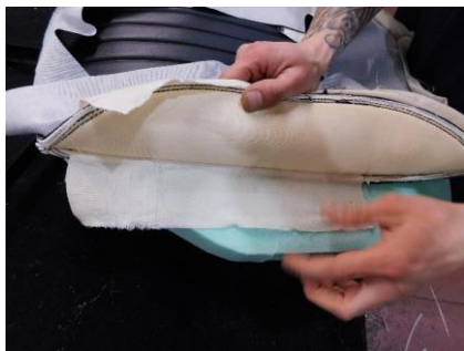
B15) Press the flaps down onto the foam. No creases.
