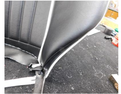
35) Staple the empty piping down onto the woods. Again tuck the side edges neatly under, pulling out any creases, then staple the bottom of the horseshoe to the tacking strip.
