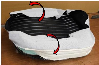
B28) Holding the frame in place, turn the assembly over, fold the rear side skirts over the sides of the assembly – as shown above right.
