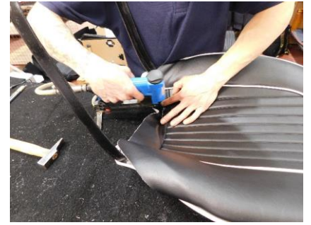
33) staple the bottom flap onto the trim strips at the bottom of the frame.
