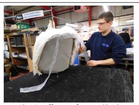
19) Trim off excess front and back. Ensure the wadding & plastic is flat and smooth. This will allow the seat cover to slide over the padding more easily.
