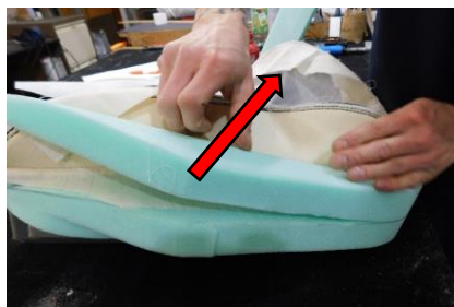
B21) Fold the sides of the cover inwards, away from the side roll foam. Lift the foam upwards & spray glue the base foam/ calico & the under side of the side roll foam. Repeat for other side.
