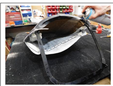
23) Place the seat on its front – the front of the seat cover hangs well away from the padding. Spray glue the back of the centre fluted area only (NOT on the horseshoe part) & on the corresponding part of the horsehair padding. Allow to dry – then repeat the gluing.
