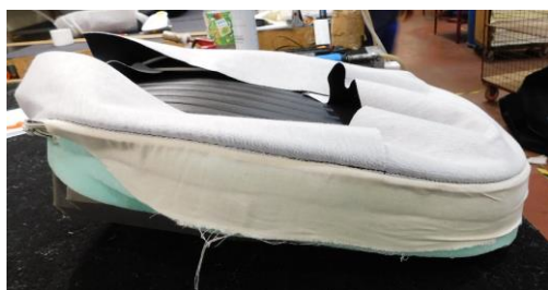
B25) Trim off any excess calico at the rear edges & your result should be as shown above.
