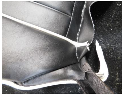
35) Staple the empty piping down onto the woods. Again tuck the side edges neatly under, pulling out any creases, then staple the bottom of the horseshoe to the tacking strip.
