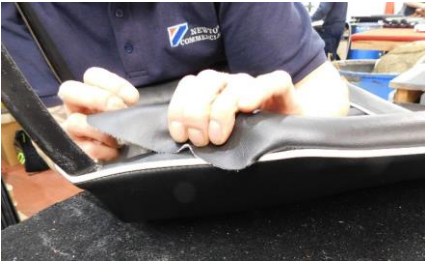
32) Tuck the side edges at the bottom of the horseshoe under to make a neat finish. Smooth them flat with your hand.
