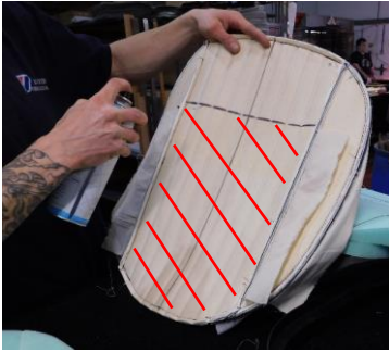
B11) Spray glue on the back of the fluted area of the cover up to the line and on the centre area on top of the base foam, to the marked lines. Where shown by the red hatch lines in the pictures above.
