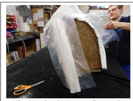
18) Place the plastic centrally over the wadding, keeping it crease free.
