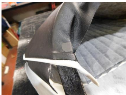
26) Having pulled the piping over the edge of the frame, the cover next to the piping can be clipped to the base frame – Repeat for the other side.
