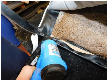
30) Staple the bottom of the flaps to the tack strip & trim off any excess.
