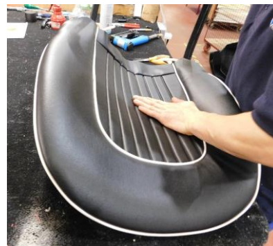
31) Lay the seat on its back. It is now time to push the two glued surfaces together. Starting at the top, push the centre fluted area down onto the padding, ensure that the flutes are vertical and that there are no creases in the horseshoe surround. The cover should be a tight enough fit to avoid any creasing. Push down firmly over the whole fluted area.
