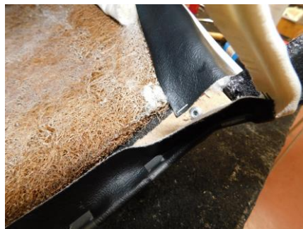
30) Staple the bottom of the flaps to the tack strip & trim off any excess.
