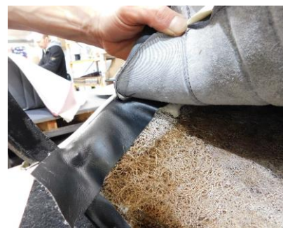
29) Glue the back of the flap & the 'horsehair' area. When nearly dry, pull the flap up over the padding & fix it into position. Repeat for the other side.
