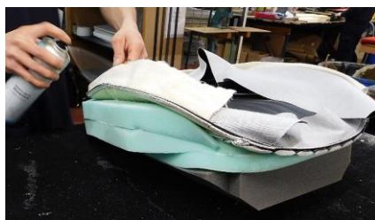
B23) Lightly spray glue the outer calico flap & then the outer vertical sides and front of the base foam/roll foam.
