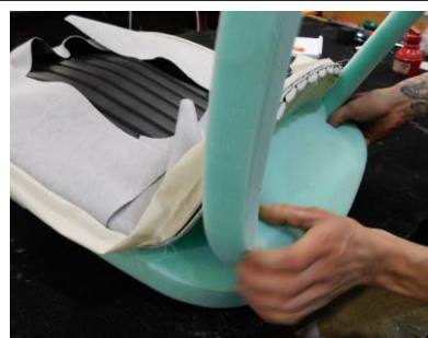
B19) Carefully position the Top Roll foam in place over the front of the Base foam with the front of the Seat Cover lifted up. Out of the way. Make sure the back edge of the roll aligns with the line marked across the front of the base pad & that all outside edges line up. When satisfied that all is well, press firmly together.
