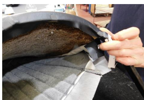
26) Having pulled the piping over the edge of the frame, the cover next to the piping can be clipped to the base frame – Repeat for the other side.
