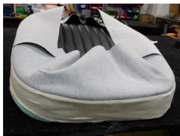
B25) Trim off any excess calico at the rear edges & your result should be as shown above.
