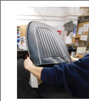
21) At the wide point of the frame, firmly grasp the seat cover where the front horseshoe joins the outer piping on both sides. (These are the weak points of the cover which need protecting so that they do not tear when pulling the cover down further) Now pull the cover fully downwards over the wide point, so that it is roughly in the correct position. Using the flat of the hand, gradually work the cover in a downwards
