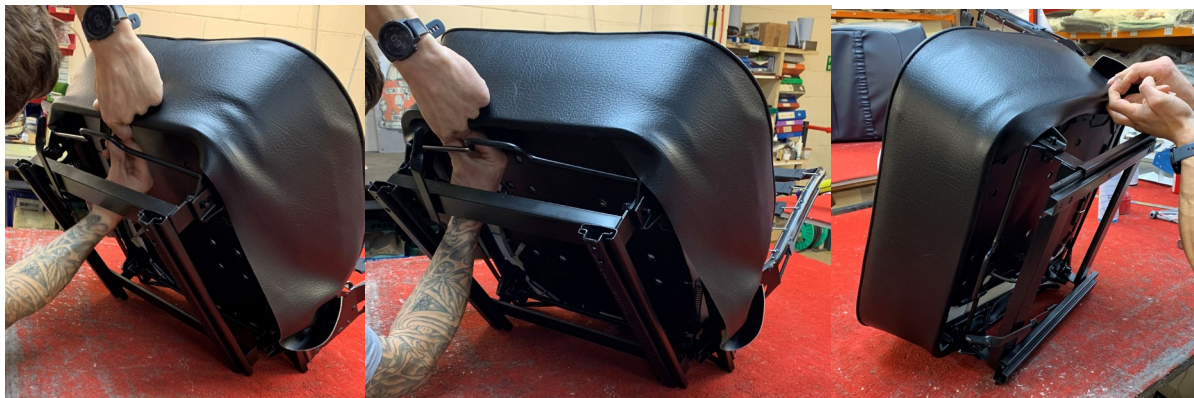
Using trim clips, attach the cover to the frame making sure vinyl is taut and crease free.
