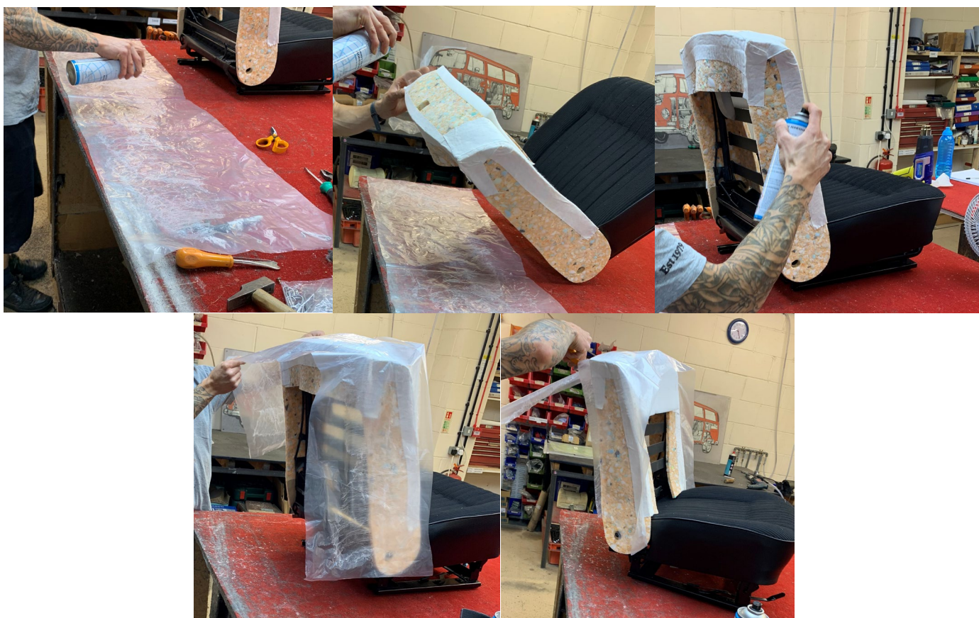
Cut a strip off the plastic bag the cover arrived in and apply some spray adhesive to one side. Apply spray adhesive around the foam being careful not to spray the cover. Place the plastic over the foam so it is taut. Trim off excess and remove plastic from the circular cut outs on the sides and the headrest slot.
