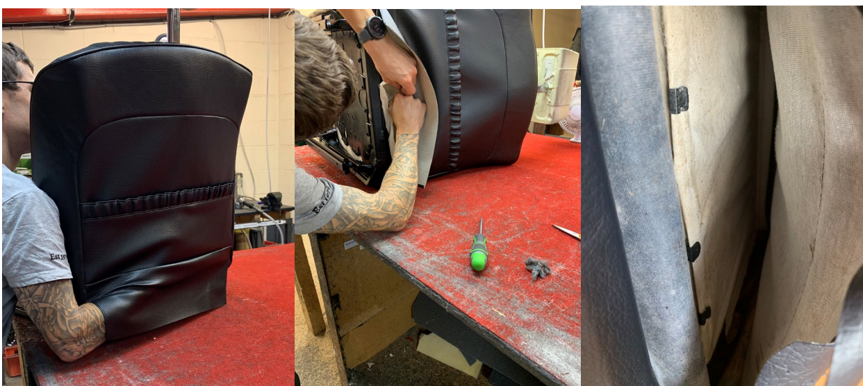
Pull the calico flap through the straps, make sure centre foam is position centrally and cover is pulled back to create the desired dip. Clip calico onto the frame with trim clips.
