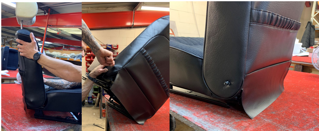
Work any creases from the sides of the cover and positioning the cover to the correct position. Once sure cover is sitting where it needs to be, cut out a hole for the stem of the reclining handle.
