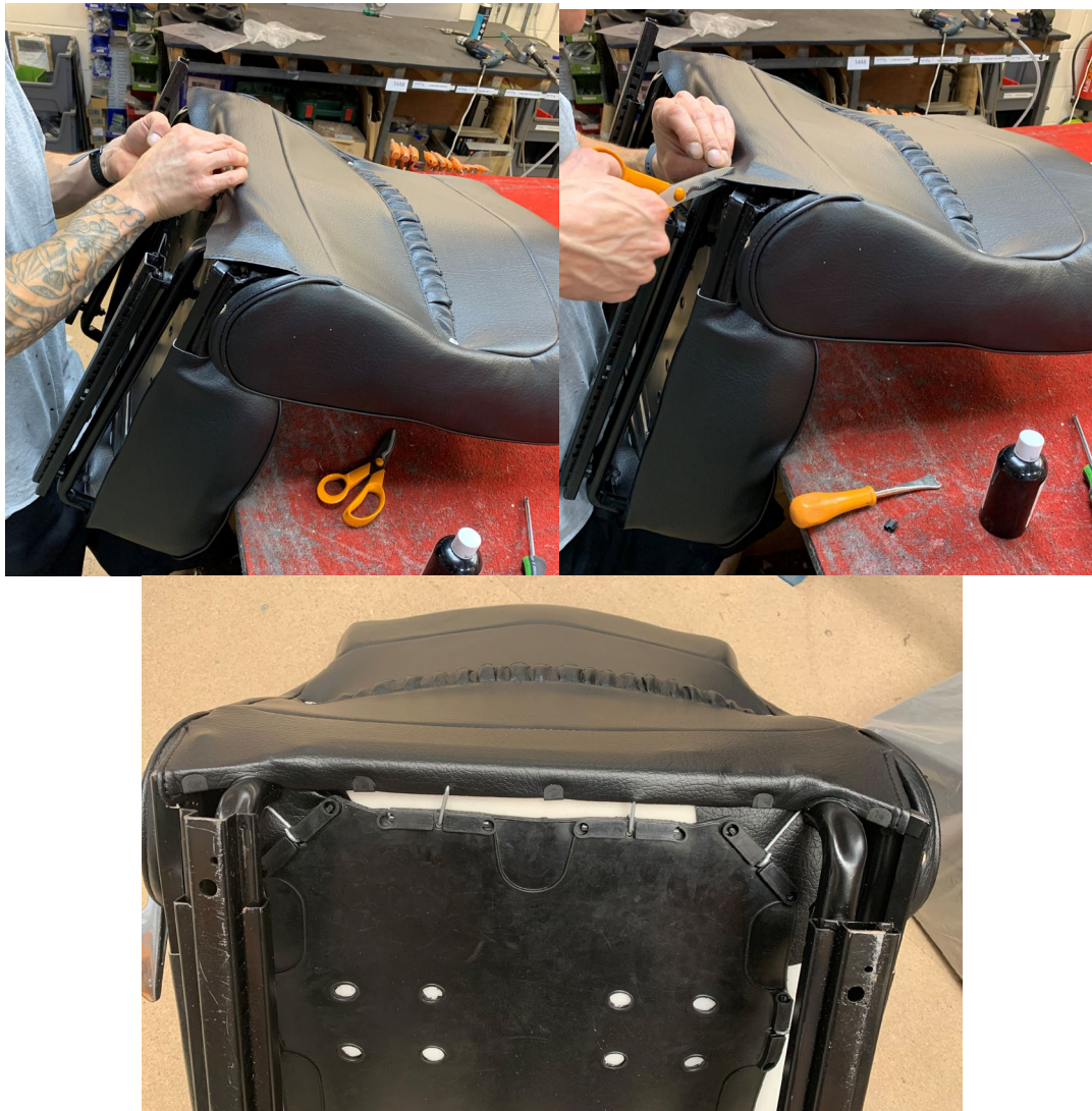
Finally, pull the rear flap taut and clip to the frame with trim clips, cut around leg of frame.
