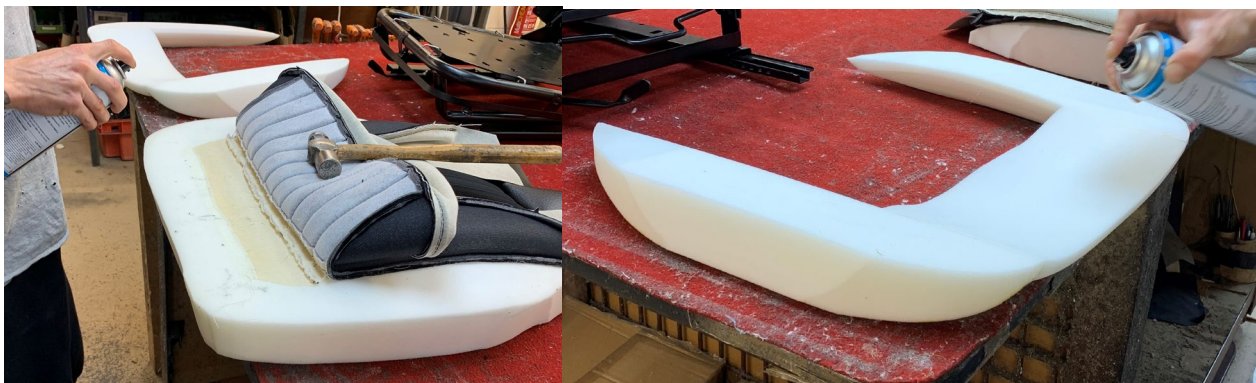
Use something heavy to hold the cover out of the way, apply spray adhesive to the remaining part of the main foam. Apply spray adhesive the underneath of the top foam.
