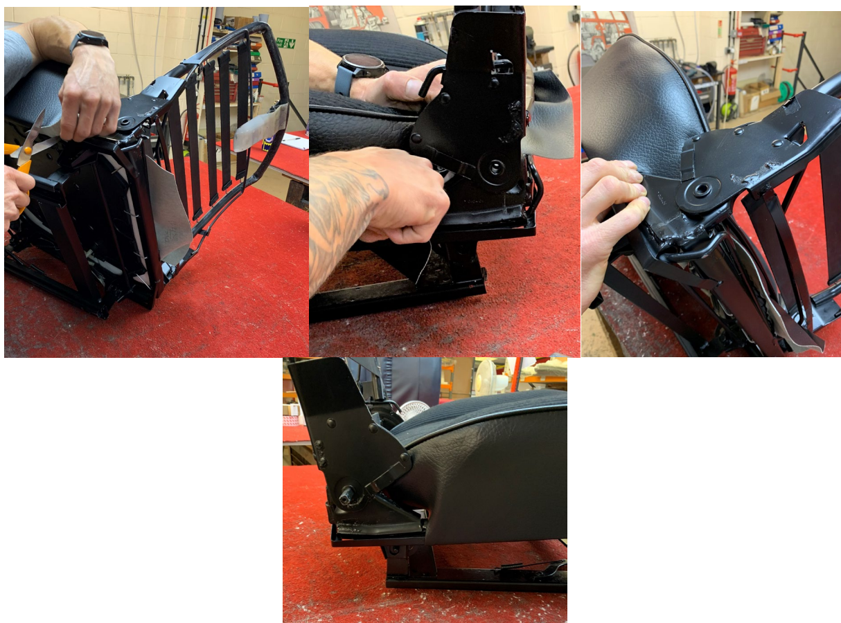
Cut into the skirt at the reclining mechanism, push through to underneath the diaphragm. Clip remaining skirt to frame.
