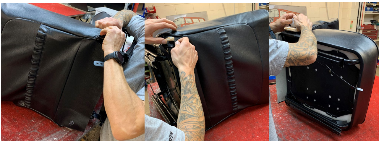
Carefully pull the squab pocket flaps over the foam and board. It may help to turn these inside out first.
