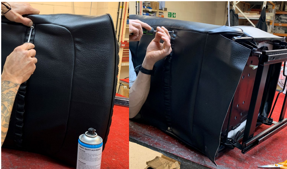
Locate the bracket on the inside of the frame and attach the two self-tapping screws into the back where the map pocket elastic is.
