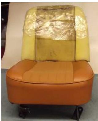
5: With the seat in this condition, the last job is to trim up the material at the rear of the frame legs. It should be simple enough to still re-adjust any clips or glue at this stage if necessary.
