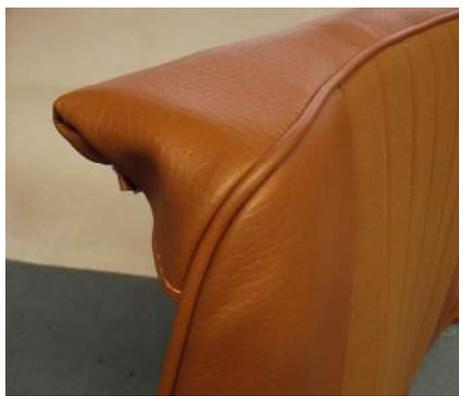
3: The top corners need to be treated like this, so that they sit neatly when the squab frame is attached to the rear bulkhead. It is usually held in place by two self tappers which pass up through the rear parcel shelf. The top rear rail of the squab frame is designed to overhang the upright lip of the rear bulkhead- the bottom will either push fit into a couple of sockets, or screw in with plastic tabs depending on the car's age.
