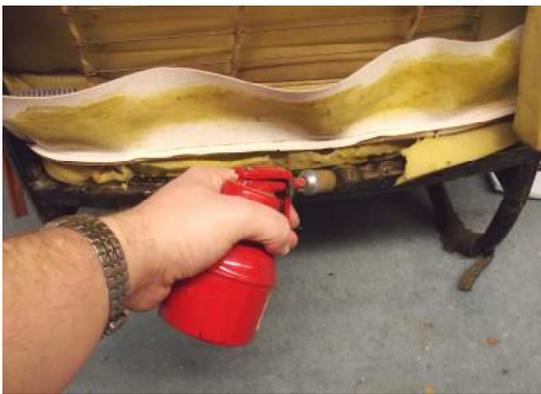
3: When you are happy with the position of the seat face on the seat foam, glue the rear flaps and the frame member.
