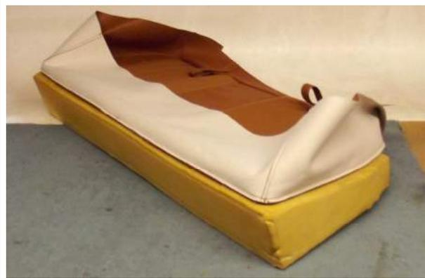
4: The base cover should be turned inside out and laid in position on top of the foam like this.
