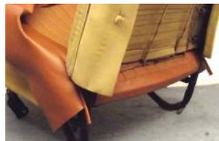
4: Having secured the cover onto the rear of the frame, the base skirt should be attached by firmly and evenly pulling down the sides, to tap in the seat clips every few inches.
