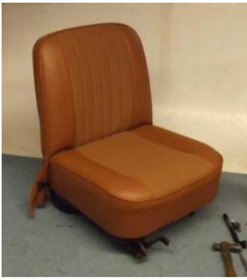
9: Slide the squab cover over the seat foam, pulling the sides right down as far as possible until the foam feels tight in the top corners.
