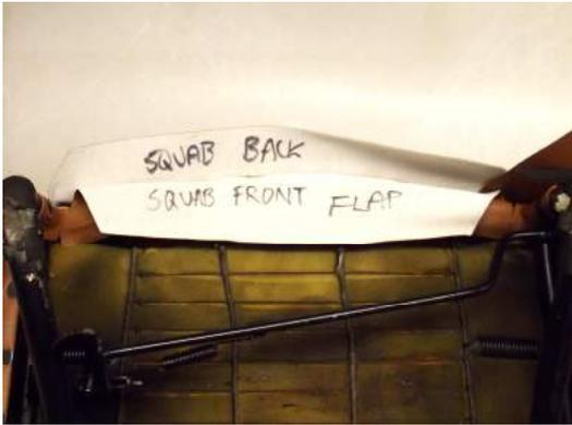
11: Ignore the seat back material for the moment. Instead glue the front flap over the bottom of the frame. Use plenty of glue here.
