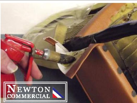
7: Glue the resulting flap. The bottom edge has been doubled over to form a neat edge. The piping will be 'lost' by tucking it under the frame later.
