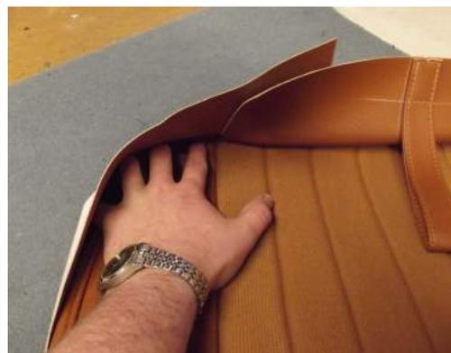
5: The base cover needs to be carefully rolled over the base foam, so that the corners at the front appear to be symmetrical/'mirror' the opposite side. The welded vinyl, or stitched cloth seat centres will largely follow the impressions which are moulded into later foams, or follow the contours made by foam topping pieces on older models. Make sure that the piping sits upright and in a straight line, all round the perimeter of the seat faces.
