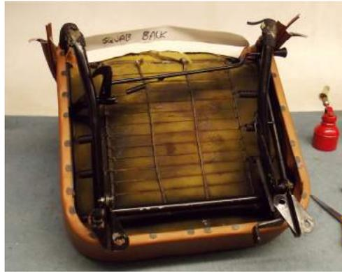
12: Trim off the excess material when the glue has cured and the flap is fixed in place. Next, give the squab skirt sides another good pull down the seat ready to stretch into position.
