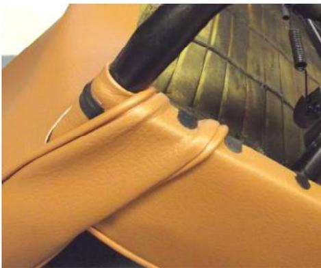
14: With the side skirts clipped into place, pull the back of the seat cover down and lightly glue it over the bottom of the frame. A few more evenly spaced seat clips are a good finishing touch- they will strengthen the covers which should now be quite taught.
