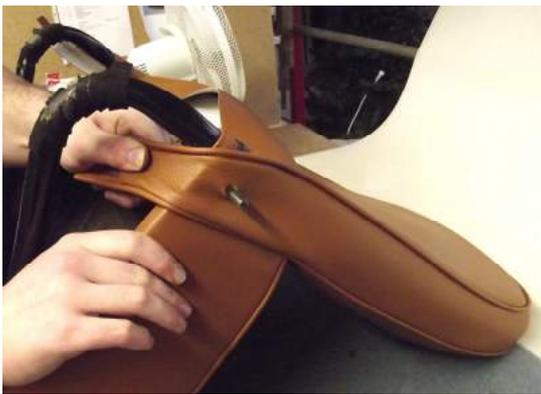
13: The side skirts can only be properly fitted with a really good tug, before clipping to the frame just in front of the legs. You will notice that this seat has an anti-tilt shaft, which requires a little more careful trimming, i.e. make sure you put the hole in the right place, because there is no going back! The exact positions of the mechanism and shaft can vary, but these were an original feature of most UK Minis built from the mid '70s onwards.
