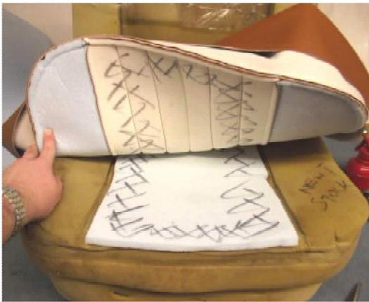
1: Begin by turning the base cover inside out and dry-fitting onto the foam. For best results, the centre of the seat should be glued to the foam. Use the shaded area as a guide.
