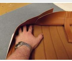
5: The base cover needs to be carefully rolled over the base foam, so that the corners at the front appear to be symmetrical/'mirror' the opposite side. The welded vinyl, or stitched cloth seat centres will largely follow the impressions which are moulded into later foams, or follow the contours made by foam topping pieces on older models. Make sure that the piping sits upright and in a straight line, all round the perimeter of the seat faces.
