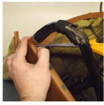
6: Turning the seat upside down, pull the excess material out of the skirt ends and clasp it tightly around the seat frame. Slit into the corner between the leg and the seat frame. The material here should be trimmed to eliminate raw edges. Apply one more seat clip right into each corner to secure.
