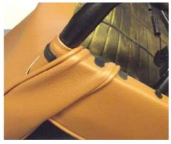
14: With the side skirts clipped into place, pull the back of the seat cover down and lightly glue it over the bottom of the frame. A few more evenly spaced seat clips are a good finishing touch- they will strengthen the covers which should now be quite taught.
