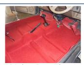
Next pull the footwell sections forward so you can correctly position the carpet as far forward on the tunnel as possible, then push the carpet firmly down until it is sitting snug over the seat mounting rails.
