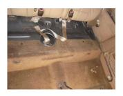
Pull the strap on the other side of the rear seat base and again remove from the car.
