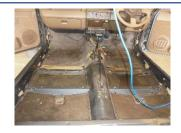
The carpet is now free to be pulled out of the car, starting at the back lift this up and over the handbrake and gear lever.
