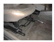
The first part of the removal process is to remove the front seats. Firstly, Slide the seat all the way back to gain access to the two T40 Torx and remove.
