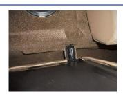
With the seat in the upright position pull forward releasing the metal tabs and remove from the car.
