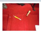
Locate all the front seat mounts with a bradle and cut the holes with a craft knife.
