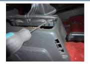
With a manual transmission the gaiter and facia are fixed in the same way with four plastic tabs, also released with a flat head screwdriver.
