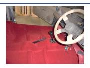
Firstly, insert the carpet into the car, pushing the front down and underneath the heater matrix. Locate the gear lever and hand brake and push through the pre-cut slots in the carpet.
