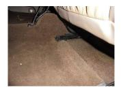
Next slide the seat all the way forward and undo the two rear T40 Torx.
