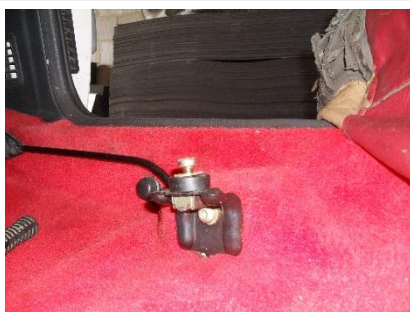
Replace rear seat mount bracket. Then replace seat belt bracket and its cover
