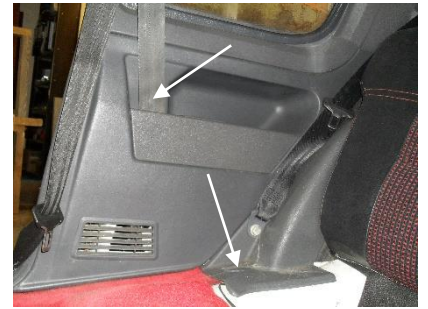
Undo the base retaining screws on the rear wheel arches. This will release the rear end of the carpet from under the plastic trim.
