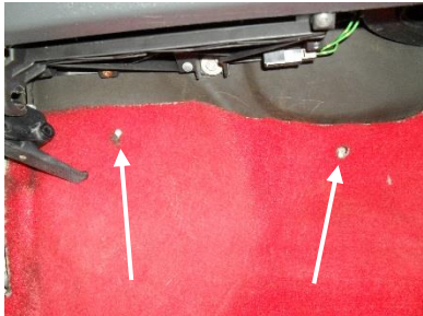
In the front foot wells, trim the carpet around the fixing studs.
