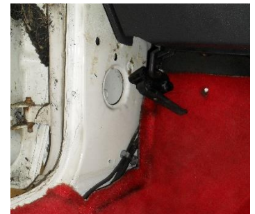
The bonnet release can rest under the dash unsupported and continue to function.
