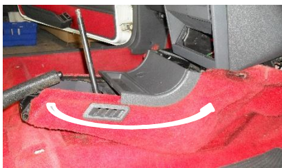
Re-fit centre console and radio. Generally refitting is the reverse of removal. See previous section of these instructions.
