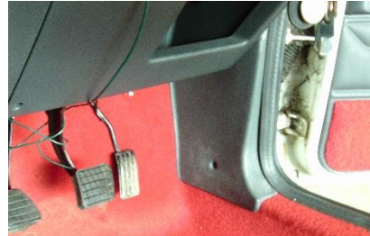
Replace Right hand scuttle panel and re-fit door seal
