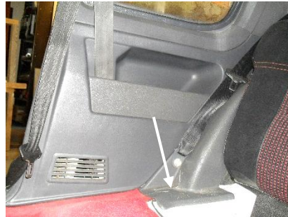
Tuck carpet under the plastic rear wheel arch cover and replace screw.
