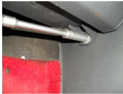
Undo the top 10mm bolt supporting the lower dash.
