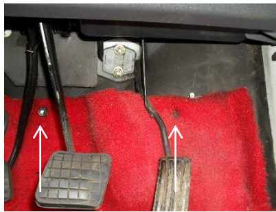
Remove the two plastic caps holding the carpet to the bulkhead on the Right Hand Side
