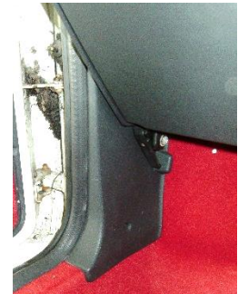
Replace Left hand scuttle panel, bonnet latch and re-fit door seal
