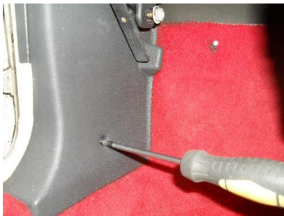
Remove the Left Hand Side scuttle crosshead screw located at the bottom of the scuttle
