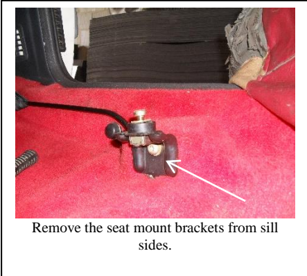
Slide Front seat rearwards remove seat front anchorage bolts (Torx T40) Repeated for other seat (Save spacers to be re-used)
