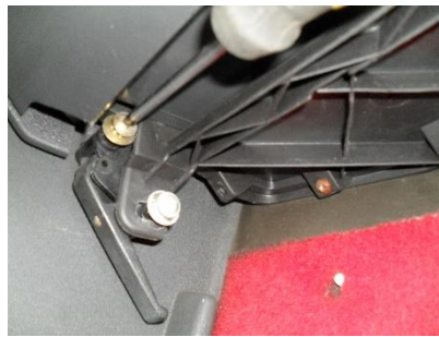
Hold the Bonnet Release in position and unscrew the two cross head screws, slide the scuttle backwards and out.
