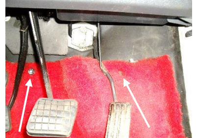
Replace all plastic retainers over the studs.
