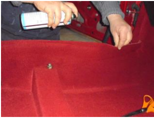
Pull back the carpet on the sills and down the inner sills, make sure the carpet is definitely pushed down in the footwells and crossmember before gluing.
