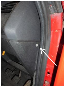
Remove the screw on the side by the door.
