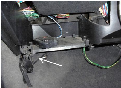
Remove the passenger side glove box and support bolt from the wheel arch.
