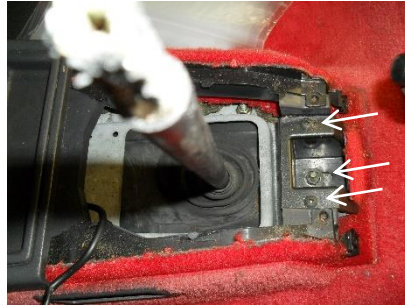
Undo the 10mm Nut and two crosshead screws and lift off bracket.
