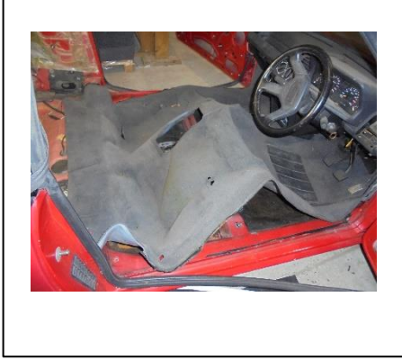
Disconnect the glove box switch, this support panel should now be free to remove from the car.
