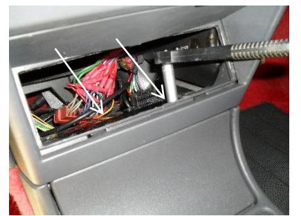
Withdraw the radio and its carrier. Unscrew and remove the two 8mm nuts.
