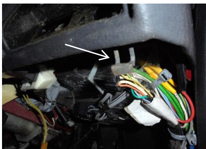
The under dash will now just be resting on this clip, unhook and remove – the dash should now be completely free.
