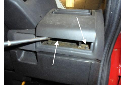
Next pry open the air vent and remove, this gives access to the last screw.
