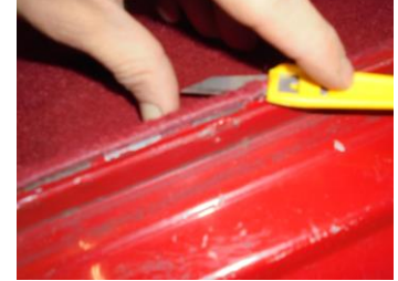
You will now need to trim the top of the carpet on the sill to create a smooth finish.
