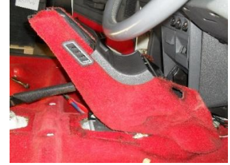
You can now refit the centre console along with the vents, gear lever assembly and handbrake surround. Refer to the removal instructions if need be as a guide on how to re-install.
