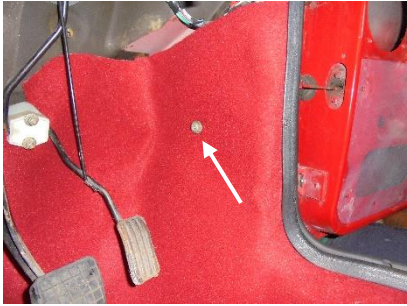
Find the driver side dash support bolt hole and make the hole with a bradawl.
