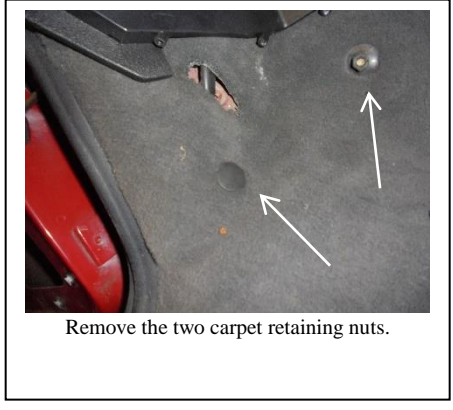
The carpet is now free to be removed. Start lifting the carpet from just behind the cross member pulling the rear ends free from under the rear quarter and wheel arch. Release the carpet from around the peddles, and pull the carpet towards the middle of the car. Repeat on passenger side. The carpet should now lift over the gear lever and hand brake to be removed from the car.
