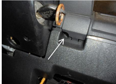
Remove the screw next to the steering column.
