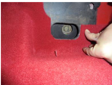
Next cut the carpet around the rear quarter air vent.
