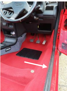
Pull back the carpet on the sills and down the inner sills, make sure the carpet is definitely pushed down in the footwells and crossmember before gluing.
