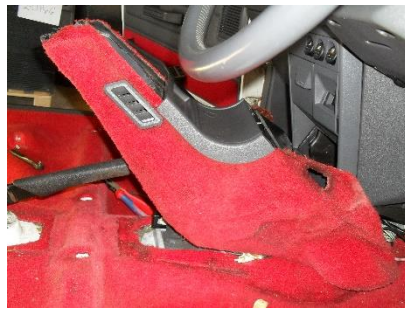
Lift the rear of the console and gently pull backwards and upwards.
