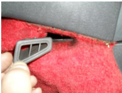
Pry and lift out the upper vents at the front of the console.
