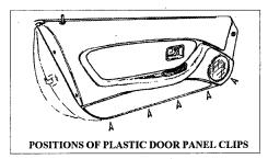
Lay the door panel on the workbench and remove any staples holding the cloth insert near the door latch hole on the back face
