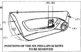
Insert the blade of the paint scraper between the panel and the door along the bottom edge. There are five plastic clips holding the panel to the door. Slide the blade along until it hits a clip then twist carefully and at the same time pulling with your free hand to release the plastic clips from the door and lift the door panel away.
