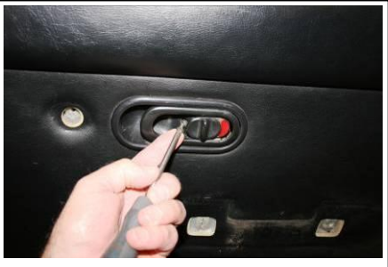
REMOVE THE PHILIPS SCREW INSIDE THE LATCH ESCUTCHEON
