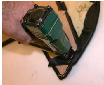
PULL THE FRONT FLAP OF THE CAPPING FORWARDS & OVER THE EDGE OF THE TRIM PANEL. STAPLE IT IN PLACE & TRIM OFF THE EXCESS. (IF YOU DO NOT HAVE A STAPLE GUN THEN USE A CONTACT ADHESIVE)
