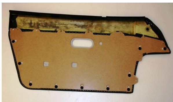
INSERT THE CLIPS INTO THE 10 KEY HOLES IN THE TRIM PANEL & 1 AT THE FRONT OF THE CAPPING
