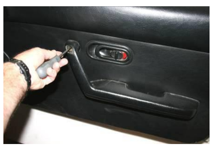
REMOVE THE SCREW AT THE TOP OF THE DOOR PULL. THE ASSEMBLY WILL NOW LIFT OFF THE DOOR.
