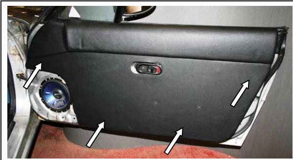
ENSURE CLIPS ARE SITTING OVER THE TOP OF THE CLIP HOLES. THEN PRESS EACH CLIP FIRMLY INTO PLACE
