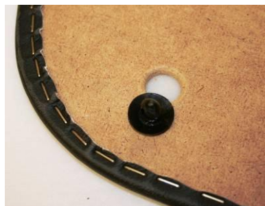
INSERT THE CLIPS INTO THE 10 KEY HOLES IN THE TRIM PANEL & 1 AT THE FRONT OF THE CAPPING
