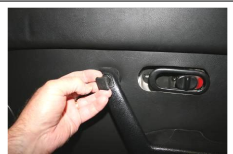
REFIT DOOR PULL/ARMREST WITH ITS THREE SELF TAPPING SCREWS IN PLACE. THEN REPLACE THE SMALL PLASTIC SCREW COVER AT THE TOP
