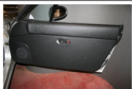
REFIT CLIPS INTO SPEAKER SURROUND MOULDING & PUSH FIRMLY INTO PLACE ONTO DOOR
