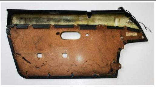
THE TRIM PANEL / CAPPING ASSEMBLY CAN NOW BE LIFTED AWAY FROM THE DOOR. BE AWARE OF ANY WIRING IF CUSTOM SPEAKERS HAVE BEEN FITTED. REMOVE ALL PANEL CLIPS.
