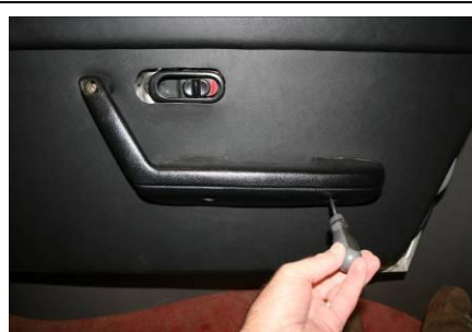
REFIT DOOR PULL/ARMREST WITH ITS THREE SELF TAPPING SCREWS IN PLACE. THEN REPLACE THE SMALL PLASTIC SCREW COVER AT THE TOP
