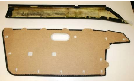
RH DOOR CAPPING & TRIM PANEL READY FOR ASSEMBLY.
