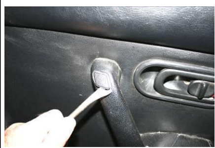
REMOVE THE PLASTIC CAP AT THE TOP OF THE DOOR PULL
