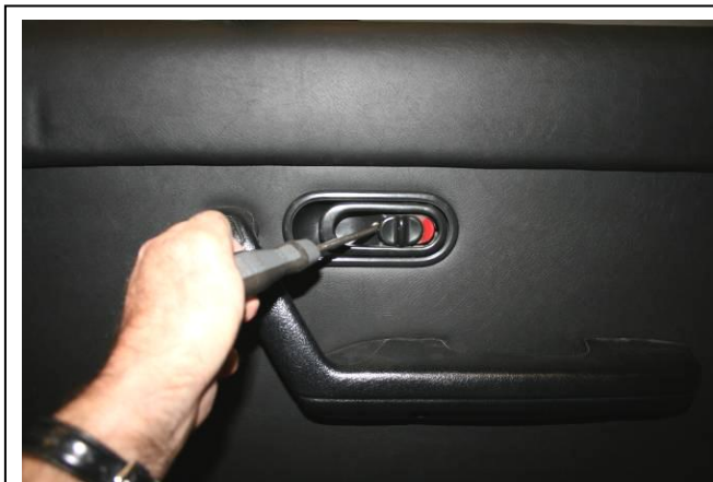
REFIT THE DOOR LATCH ESCUTCHEON & SECURE WITH ITS SCREW
