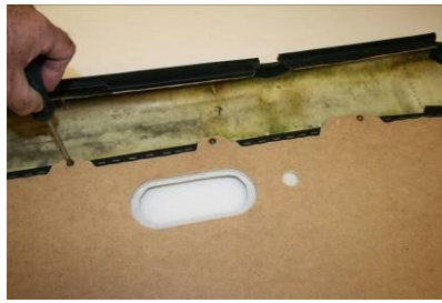
LINE UP THE CAPPING WITH THE TRIM PANEL & FIX TOGETHER USING THE SMALL SELF TAPPING SCREWS
