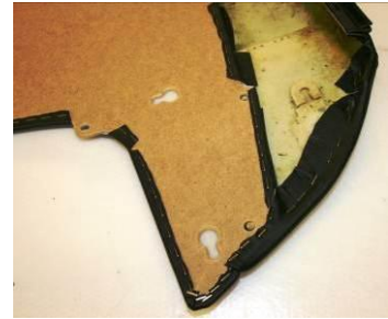
PULL THE FRONT FLAP OF THE CAPPING FORWARDS & OVER THE EDGE OF THE TRIM PANEL. STAPLE IT IN PLACE & TRIM OFF THE EXCESS. (IF YOU DO NOT HAVE A STAPLE GUN THEN USE A CONTACT ADHESIVE)
