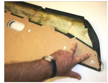
PUSH THE TWO FRONT PLASTIC POSTS THROUGH THE HOLES. (THESE CAN BE MELTED OVER USING A HOT SOLDERING IRON)
