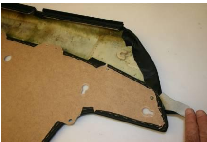
PULL THE FRONT FLAP OF THE CAPPING FORWARDS & OVER THE EDGE OF THE TRIM PANEL. STAPLE IT IN PLACE & TRIM OFF THE EXCESS. (IF YOU DO NOT HAVE A STAPLE GUN THEN USE A CONTACT ADHESIVE)
