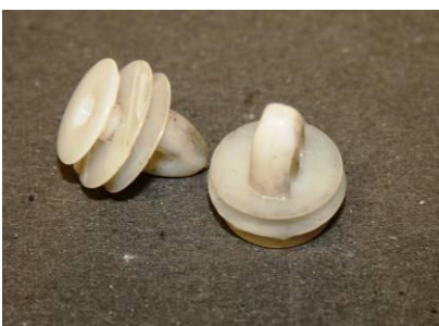
ORIGINAL FACTORY PANEL CLIPS. IF YOURS ARE IN GOOD ORDER, THEY CAN BE RE USED
