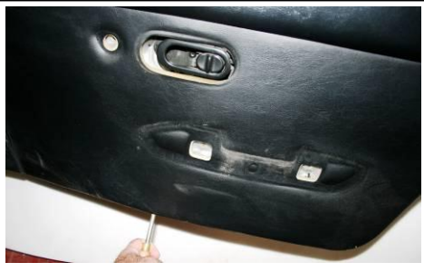
PLACING A TRIM REMOVAL TOOL (OR A FLAT BLADE SCREWDRIVER) BETWEEN THE TRIM PANEL & THE DOOR, RELEASE THE CLIPS DOWN THE FRONT, BACK & ALONG THE BOTTOM OF THE DOOR, USING A LEVER ACTION.
