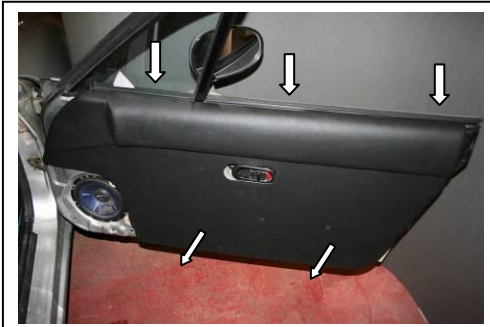
LOCATE THE DOOR ASSEMBLY ONTO THE TOP OF THE DOOR. KEEP THE BOTTOM EDGE AWAY FROM THE DOOR
