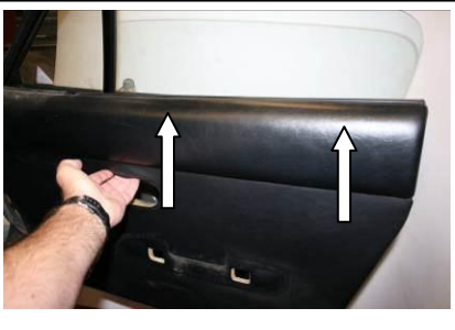
LIFT THE PANEL ASSEMBLY UPWARDS TO DISENGAGE THE TOP EDGE OF THE CAPPING FROM THE DOOR
