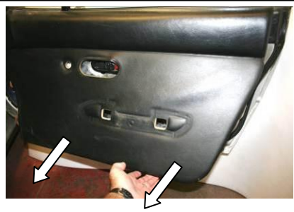
WHEN ALL CLIPS ARE DISENGAGED, THE PANEL & SPEAKER COVER CAN BE PULLED AWAY FROM THE DOOR
