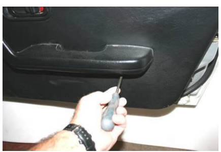
WITH A PHILIPS SCREWDRIVER, REMOVE THE TWO LARGE SELF TAPPING SCREWS UNDER THE ARMREST
