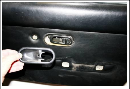
LIFT THE ESCUTCHEON OVER THE DOOR LATCH
