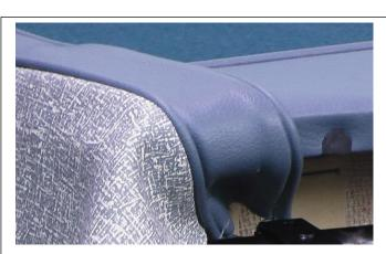
7) Maintaining downward pressure, fold the bottom of the side skirts around & under the lower frame. (You will feel the metal tabs inside the pockets – once these are bent round the frame in front of the leg, the squab cover is held in place)
