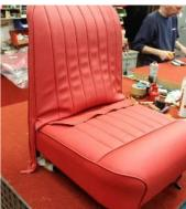
5) Slide the squab cover down over the squab assembly. *Important Note*; Firmly grip the cover at the bottom of the side piping. (This is the strongest area of the squab cover & will avoid damaging the cover under tension). Pull the cover fully down so that it sits as in the picture on the right.
