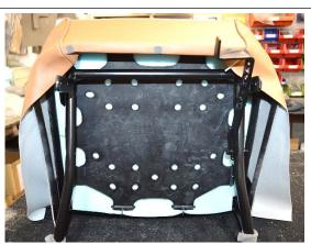
10) Pull the front of the skirt evenly over the front roll & clip in place along the straight portion of the front lower frame.
