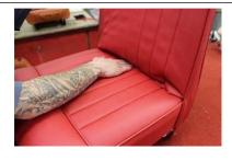
8) With the sides now anchored, feed the front flap & lower portion of the fluted section under the padding & behind the diaphragm. Push it so that it lies flat behind the diaphragm. Once in place properly it will stay in place without the need for any glue.
