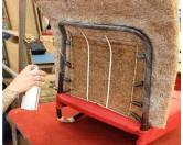
1) Take the Horsehair pad (From Squab Padding Kit – SF666) & position it at the front of the squab frame centrally, resting on the base cover. Using a Marker Pen, mark around the outside of the frame.
