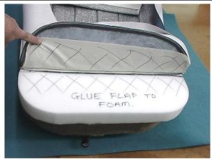
5) With the seat cover positioned centrally & glued in place behind the front roll, glue the Calico Flap to the base foam. (Glue flap & foam where indicated)
