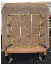
2) Fold the padding around the frame taking care at the top corners to fold as neatly as possible. (Note; achieving smooth corners at the top is most important). Trim off excess where the padding has to be gathered in on the inside of the corners so that you are left with no lumps at the back
