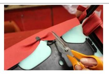
11) Pull the back down over the rear frame cross member. Clip it in the centre & work outwards, snip the flap to clear the diaphragm hooks.
