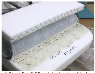
6) Take the Front Roll Foam & glue along the straight edge. Glue along the back edge of the Calico Flap (See above)
