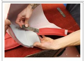
4) At the bottom of each side skirt on the squab cover is a pocket which holds a metal tab (These should be available to re-use from you old seats – if so, make sure they are flat) Slide a tab fully into each pocket.
