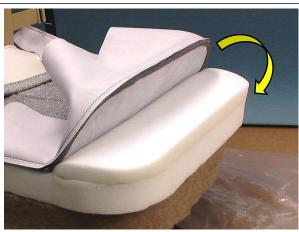
8) Bring the Roll Foam down onto the Base Foam – Make sure the outside edges line up first, then press the foams together.
