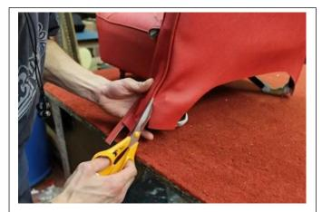
6) With the cover pulled down at the sides, feel inside for where the bottom frame meets the leg, cut with scissors on the back, next to the piping, to about 5mm of this point on each side.
