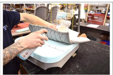
4) Lay the base cover on the foam, the piping join where the front roll meets the fluted section should line up with the marked line on the base foam. Make sure the cover is placed centrally. (It may help to mark the mid-point on the cover to give a reference point) The rear of the cover should lay over the rear of the base foam. Push the rear flap under the squab diaphragm.
