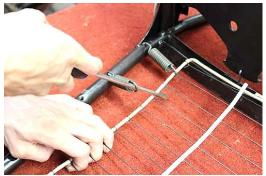
1) Strip off old seat covers, foams & diaphragms from the frame. Inspect the frame, clean, check for damage, repair and repaint as necessary. Fit new base diaphragm (C705) and squab diaphragm (C708).
