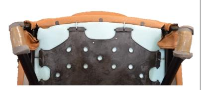
12) Fit another 3 or 4 clips along the rear flap & tuck the raw edge in between the frame & the base foam to give a neat finish.
