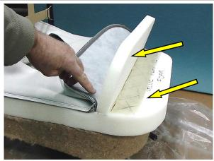
7) Once the glue is dry, position the Front Roll Foam with its top edge in line with the edge of the Calico and cover join.
