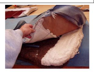
Again using the screw driver, remove the old cover from the frame. When taking the old cover off, note how any wadding or felt is positioned over the horse hair pad.
