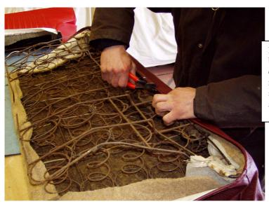
Lay the seat cover over the frame, centralize and begin by turning the skirt over the two front corners. Pull the skirt over all edges and then Hog ring through the edges to the second bar in of the seat frame. You will need to pull the cord to actually tighten the skirts at either end.
