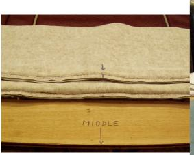
Inspect the spring frame for any damage and repair as necessary. If the horsehair looks a bit thin in places it may be a good idea to cover it with a layer of felt. Allow enough felt to actually fall over the sides as shown here to give you smooth corners and edges.
