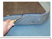
Remove the various screws holding the seat brackets and locking flap. The using a flat screw driver remove the tacks holding the backboard to the seat frame.
