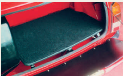
SINGLE TANK BOARD 1980-92 (7.5 GALLON TANK) Complete board CK954 Overall width of board 29" (737 mm) Pre fuel injection cars
