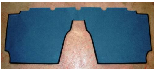
THE BULKHEAD CARPET IS FITTED AS SHOWN WITH ITS CENTRE OVER THE TUNNEL. THE BOTTOM EDGE SITS ON TOP OF THE FLOOR MATS & IS HELD IN PLACE USING 4 PLASTIC STUDS (YOU SHOULD HAVE NO DIFFICULTY LINING UP THE HOLES). THE TOP EDGE IS POSITIONED UNDERNEATH THE FRONT EDGE OF THE REAR LOAD AREA CARPET. BOTH ARE HELD IN PLACE WITH 5 PLASTIC STUDS
