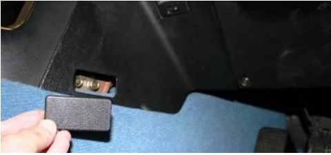
REPLACE THE 2 SCREWS & THE PLASTICCOVERS ON EACH SIDE OF THE CONSOLE.
