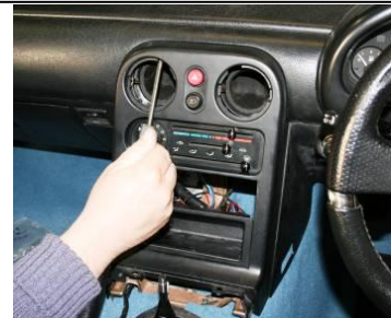
RE-FIT THE FRONT PANEL. PUSH THE ELECTRICAL PLUG IN PLACE AT THE BACK OF THE SWITCH. REPLACE THE PANEL & RE-FIX THE 2 SCREWS UNDER THE AIR VENT HOLES.
