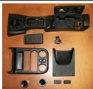
CLEAN ALL THE CENTRE CONSOLE PARTS
