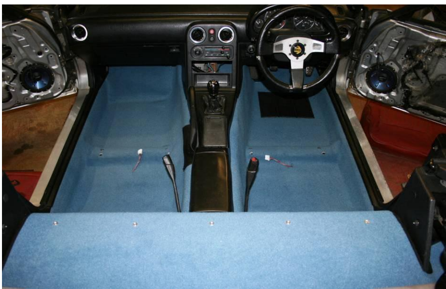
REFIT THE ASHTRAY, GEAR KNOB & ANY RADIO EQUIPMENT. YOUR CARPET SET FITTING IS NOW COMPLETE. FINALLY REFIT YOUR SEATS (DON'T FORGET THE ELECTRICAL CONNECTIONS UNDERNEATH) & RECONNECT THE BATTERY. YOUR CAR IS NOW READY TO DRIVE.
