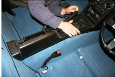
TURN THE CONSOLE THE RIGHT WAY UP. LOCATE THE REAR END FIRST OVER THE LEVERS, THEN LOWER THE FRONT END PASSING THE GEAR LEVER THROUGH ITS GAITER. REFIT THE 5 CONSOLE SECURING SCREWS.
