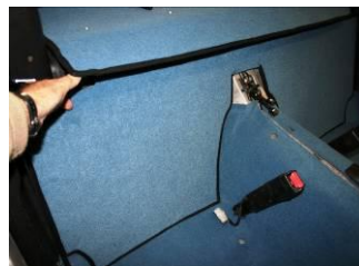
THE BULKHEAD CARPET IS FITTED AS SHOWN WITH ITS CENTRE OVER THE TUNNEL. THE BOTTOM EDGE SITS ON TOP OF THE FLOOR MATS & IS HELD IN PLACE USING 4 PLASTIC STUDS (YOU SHOULD HAVE NO DIFFICULTY LINING UP THE HOLES). THE TOP EDGE IS POSITIONED UNDERNEATH THE FRONT EDGE OF THE REAR LOAD AREA CARPET. BOTH ARE HELD IN PLACE WITH 5 PLASTIC STUDS
