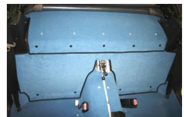
THE BULKHEAD CARPET IS FITTED AS SHOWN WITH ITS CENTRE OVER THE TUNNEL. THE BOTTOM EDGE SITS ON TOP OF THE FLOOR MATS & IS HELD IN PLACE USING 4 PLASTIC STUDS (YOU SHOULD HAVE NO DIFFICULTY LINING UP THE HOLES). THE TOP EDGE IS POSITIONED UNDERNEATH THE FRONT EDGE OF THE REAR LOAD AREA CARPET. BOTH ARE HELD IN PLACE WITH 5 PLASTIC STUDS
