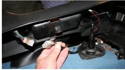
OFFER UP THE CENTRE CONSOLE ASSEMBLY & RE-CONNECT THE 2 PLUGS
