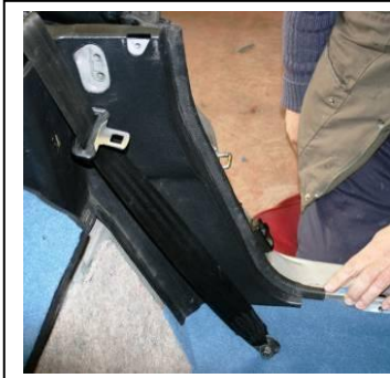
RE-FIT REAR DOOR SEALS. ENSURE THEY LINE UP AT THE TOP
