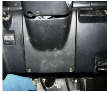
RE-FIT THE PLASTIC PANEL UNDER THE STEERING COLUMN.
