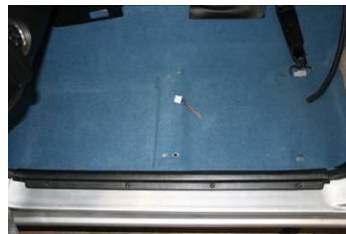
SILL STRIP RE-FITTED.
