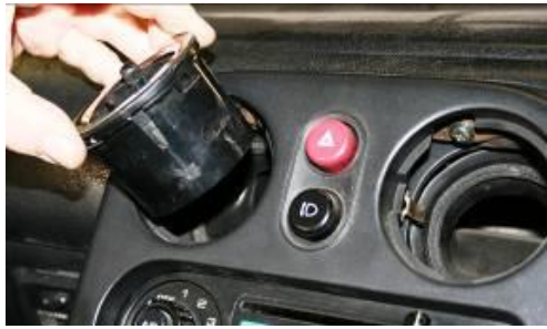
REPLACE THE AIR VENTS
