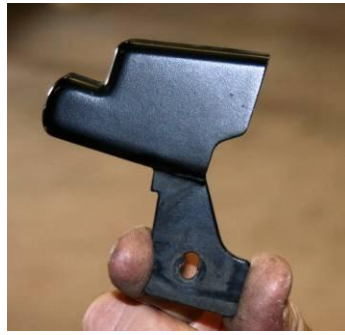
RE-FIT LEFT & RIGHT CAPPINGS. EACH FIXED IN PLACE WITH A CROSS HEAD SCREW & A "LIFT THE DOT" SCREW. (USE A 10mm SPANNER TO TIGHTEN).
