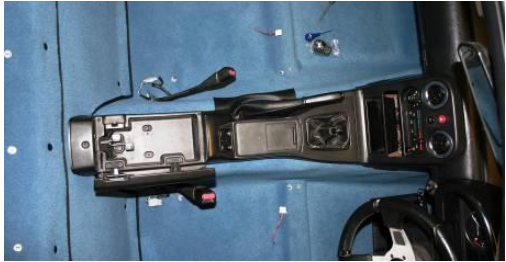
TURN THE CONSOLE THE RIGHT WAY UP. LOCATE THE REAR END FIRST OVER THE LEVERS, THEN LOWER THE FRONT END PASSING THE GEAR LEVER THROUGH ITS GAITER. REFIT THE 5 CONSOLE SECURING SCREWS.
