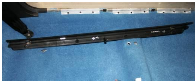
POSITION THE PLASTIC SILL STRIPS OVER THE SILL JOINTS. THIS WILL COVER THE PLASTIC CARPET CLIPS (IF FITTED) & THE ENDS OF THE DOOR SEALS. MAKE SURE THE SMALL METAL CLIPS ARE IN PLACE
