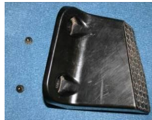
RE-FIT THE DRIVERS FOOT REST. (10mm SOCKET)
