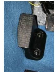
RE-FIT THE DRIVERS FOOT REST. (10mm SOCKET)
