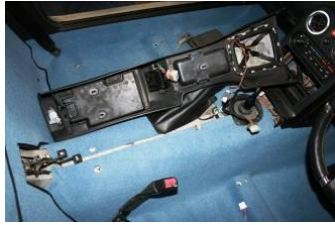
OFFER UP THE CENTRE CONSOLE ASSEMBLY & RE-CONNECT THE 2 PLUGS
