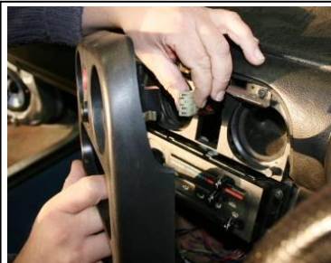
RE-FIT THE FRONT PANEL. PUSH THE ELECTRICAL PLUG IN PLACE AT THE BACK OF THE SWITCH. REPLACE THE PANEL & RE-FIX THE 2 SCREWS UNDER THE AIR VENT HOLES.
