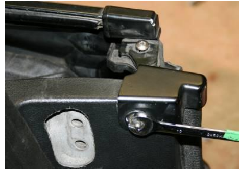
RE-FIT LEFT & RIGHT CAPPINGS. EACH FIXED IN PLACE WITH A CROSS HEAD SCREW & A "LIFT THE DOT" SCREW. (USE A 10mm SPANNER TO TIGHTEN).
