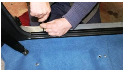
RE-FIT THE 4 CROSSHEAD SCREWS
