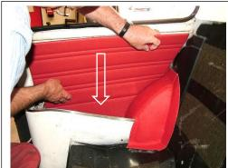
Insert the panel down into the pocket so that the top edge of the panel sits just above the metal channel and parallel to it.
