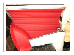
This picture shows the Rear Quarter panel fitted correctly, ready for the rear pocket liner & rear seat to be fitted.
