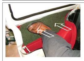
This illustrates the amount of pressure that may be needed. It can be easier to use foot rather than hand power because you can brace yourself against the opposite side of the car more readily. If using this method, please ensure you use a clean piece of felt or foam to avoid any damage to the quarter panel. (Also good to have some scrap felt or carpet across the rear seat pan, as there are lots of sharp edges in the back of a Mini without the rear seat fitted.)
