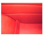
Next fit the Rear Pocket Liner. Fold it to shape along the crease lines. It should be a very tight fit against the metal bin and the Rear Quarter Panel. We would recommend using a hammer handle to provide force along the bottom edges of the pocket liner, as fingers alone do not usually provide enough of a solid contact to push the liner into place. If ashtrays are fitted, use a sharp knife to cut out the aperture then fit the ashtray.
