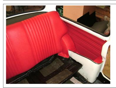
The rear seat squab assembly can now be fitted into the car.
