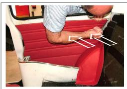
Apply *considerable* pressure to the panel (At approximately the same height as the door lock) towards the outside of the car.
