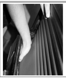
So that it sits in front of the spacer, you will need to pull the bottom of the panel forward. This can be difficult and will need some force. However by grasping it with one hand inside the bin to locate it, and pushing the panel down from its top with the other hand, it will fit quite snugly between the spacer and the drain pipe.
