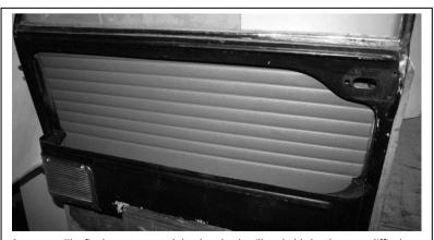
8: The final corner around the door latch will probably be the most difficult part of the board to turn under. It really does need a good push to go under the lip. You will find once it has, your door should look something like this, awaiting only the fillets and liner to complete the trim. These panels are held in by tension alone, the fillet panels keep them curved to shape, and stops them moving inside the door.
