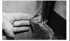
1: First of all, check that you are happy with the condition of your doors. Check that there is sufficient clearance between the ends of the door bins and the door skin, and that there are no projecting sharp edges. Generally if you can get your fingers between the two this should be fine.
