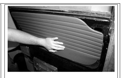
6. With the panel inserted correctly at the front end of the door frame, if you have not already got the opposite end of the panel down into the bottom of the door frame, push it down also. Take care to support the middle of the board pushing the panel so that it bows to the shape of the door, to protect the material from snags.
