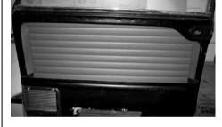
15: This shows how the fillets and door panel should look when correctly fitted. The horizontal lines of the door design should be level, the fillets are vertical and fill the door gaps nicely.
