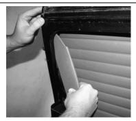
12: It does not matter which order the fillets are fitted in- we are fitting the front fillet to a Right-hand door here. Insert it with the straight edge to the door by pushing it up into the slot made for it.
