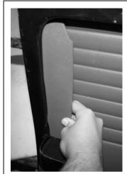
When the fillet is running straight against the inside of the door, bring it down the slot so that it sits level on to the top of the ledge that forms part of the door bins.
