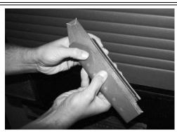
10: Prepare the fillet panels by folding over the flaps to stretch them into the shape they hold when fitted. The flaps are creased into the fibreboard material so this is quite simple. The riveted flap with the curved edge is wider, and on each fillet this is the part that bears against the door panel to help it keep its shape. The straight edge with the small flap is the side that bears along the vertical edge of the inner door frame.
