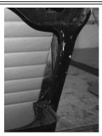
9: The fillet panels tidy the area around the ends of the inner door frame, basically filling the gaps- hiding the door latch mechanism at one end, the hinges at the other, and the myriad of pipes that the sliding window channels drain into. Make sure before fitting that the pipes and any other obstructions are well back into their recesses.
