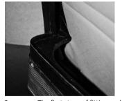
2: The first stage of fitting each new panel is to slot the panel into place carefully behind each end of the door bins, as shown here. The door panel should be held in by an equal amount on each side.
