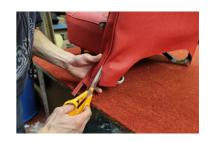
There is a pocket at the bottom of the side skirts where you can insert the metal plate. Start to pull the squab cover over the frame and go down as far as possible. Pull only on the pipings and not on the face or the back panel which could split the material. Once the cover is right down, turn the bottom of the skirt under the frame. The metal plate will turn under to secure the skirt.
