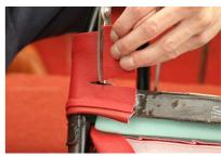
The end of the skirt needs to be trimmed and glued around the vertical tube as shown here.
