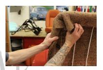
The horse hair pad needs gluing to the squab frame. Apply adhesive to the front tube and the corresponding area of the pad. The bottom of the pad should sit just above the base cover. Apply more adhesive to the whole of the reverse side of the pad as well as the tube. Turn the edges of the pad around the frame and at the top corners squeeze to gather the pad to create a rounded corner.
