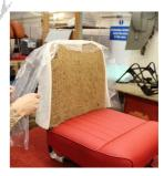
Trim the excess material from the corners of the pad to create a soft rounded corner. The white wadding can now be folded and glued to the top surface of the pad and the finally a strip of plastic can be glued over the top of the wadding. This plastic will help you slide the squab cover down more easily.
