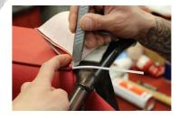
You can now secure the skirt of the cover to the frame with the clips. Start at the front with one clip and then with a couple of clips on either side so that you can check to see that the alignment is correct. When satisfied, apply more clips. Using a very sharp knife, slit the piping material to release the piping cord inside. By removing this cord the three layers of material will be reduced.
