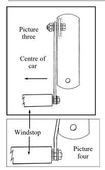
Please read these instructions carefully to familiarise yourself with this operation. It is not difficult and should take you about half an hour. It will be necessary to lift the "T" bar away from the bulkhead to fit the brackets. You will not have to remove it completely.
