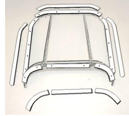
Trim strips in position on the Squab Frame
