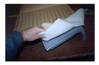
Trim and clip/ glue the sides and bottom flap to the back of the padding frame.
