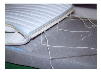
Take the new base cover and insert the four trim wires from your old seat cover into the calico hoops.
