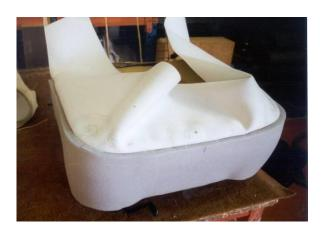
j) Fold the base skirt down over the base wrap all around this will be a tight fit and will require pulling firmly. Start at front middle – clip the cover onto frame. See Picture 6 to the right
