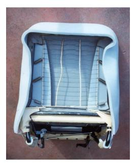
If your seat is fixed – re-tension and clip the sides. Then fix front and rear flaps as shown in instructions for squab.
