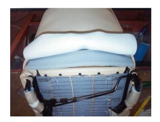
m) Insert an edge softener foam along the bottom of the frame and then pull the back cover over the frame and clip in place. **See picture 11 above**. Use your other seat as a reference to see how it is trimmed.
