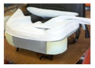
i) Glue a base wrap (use soft felt or approx. 12mm thick foam.) over the whole of base frame / foam up to the top of the calico flap. See picture 5 to the right
