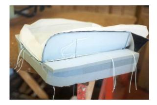
f) Looking form underneath the foam, you now have eight strings along each side of the foam directly under the edge of each side roll. These strings can either be tied securely over another wire. Which then can be tied or hog ringed to the diaphragm or tied directly onto the wire base diaphragm. This will hold the centre-fluted section of the seat firmly onto the foam and the whole assembly onto the frame
