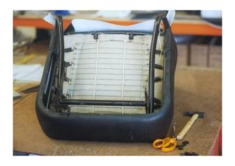
$\mathbf{k}$ ) At the rear the cover can be glued and clipped around the tubular part of the frame.
