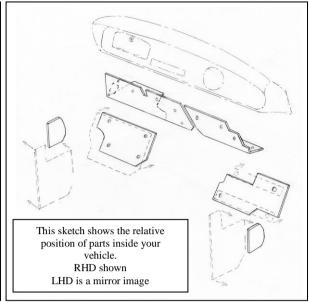
Originally the normal method of sound insulation for Herald/Vitesse was glass fibre wool encased in a polythene bag. This was roughly shaped to fit the required area & simply stuffed behind the trim panel. It was to be found in the doors, rear quarter area, under the gearbox cover & under the dash area (Held in place by the fibreboard under dash trim panel).
