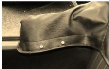
Using the punch and anvil supplied, and removing the cover to a work area again, fit two sockets on each side in the positions you have marked. Refit the cover again for the next and final stage.
