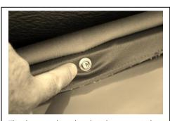
The three studs and sockets have now to be fitted. These will follow, as related earlier, the three positions of the screws that retain the back of the hood proper. The cupwashers are effectively replaced by the D. dot stud fixings. As mentioned before, If the screws do not fit well within and flush to the bottom of these stud fixings, or are domed, the screws must be replaced. Please refer to page 2 for advice.
