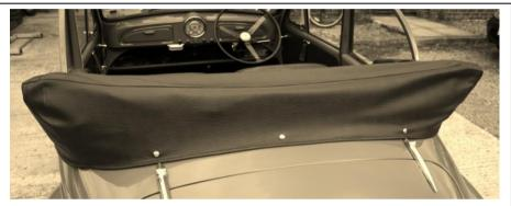
It is next necessary to fit the three durable dot fastenings across the rear of the car, after which the Hood Cover should look like this. In order to mark the positions of the three D. dot sockets, leave the Hood Cover affixed by the two Lift a dot fastenings that you will have already fitted. These should be capable of pulling the material reasonably tightly across the back of the car, so that it can hold a shape like the above, for the correct positions to be marked.
