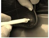
When you are happy with the loose fitting Hood Cover, pull the exterior front corners over the Lift a dot stud at the back of the rear window. Mark an identical point on each side. This will be used to locate the new lift a dot fastenings.
