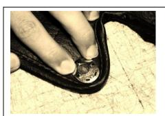
Having marked a point on each side, remove the Hood Cover to a work area or flat surface, and position the two Lift a dot flat plates, so that the points marked lie in the middle of the large hole in the plate. You will notice the plate is slightly elongated; the wide end of the plate points to the corner/front of the car.
