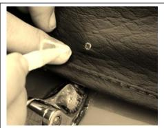
When the studs have been fitted to the body of the car, you next need to mark the positions of the D. dot sockets on the face of the hood roll cover, preferably with a white pencil. Make three holes with a spike or bradawl, just large enough for the stem of the chromed buttons to be a tight fit, as shown.
