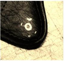
Using a fine paint pen or a point of soluble white pencil, hold the plate in position firmly and mark the four points that receive the prongs of the Lift a dot tops, and the large central stud hole.
