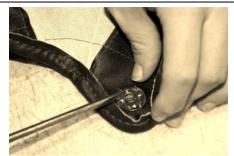
You will notice the plate isn't quite flat; it should be slightly convex. The bowled side, or the inside of the curve, should face inside the Hood Cover towards the car, and away from the visible material. Bend the prongs outward slightly using a suitable flat, hard tool.
