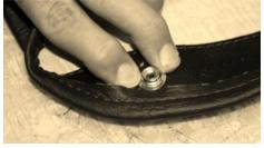
Satisfied with the location of the button, place it face down into the anvil. Push one of the sockets onto the stem, and centre firmly in the anvil. Next it is necessary to use the special punch supplied with the anvil, which in effect will rivet either stud or socket fixings to the buttons.
