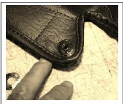
Having made the necessary holes in the Hood Cover, position the Lift a dot tops, making sure the hole cut from the material matches the size of the hole in the top.
