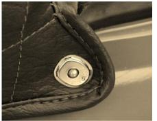
Once the prongs have been bent down a little, they can be tapped flat against the plate with a pin hammer. The two Lift a dot fastenings should then be capable of holding the Hood Cover in shape across the rear of the car, and should fit flat, as above.
