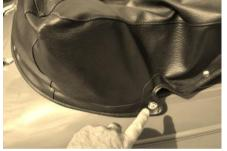
This picture shows the eventual position of the side of the Hood Cover- the ends cover the hood frame and lie inside the rear side windows. Trial fit, and centre, the new Hood Cover, over the hood assembly.
