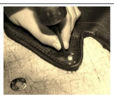
Use a small punch and a hammer to carefully cut the stud hole out of the material, as marked. The Tonneau Spike supplied can now be used to perforate the prong positions as also marked previously, with a sharp tap from a hammer. Take care to do this on an old work surface!
