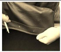
Holding the cover over the frame in such a way that you are happy with its appearance and fit, nip the hemmed edges together. Mark two positions for the sockets, on the material facing inside the car, on each side of the cover. These should be about 6 inches apart.
