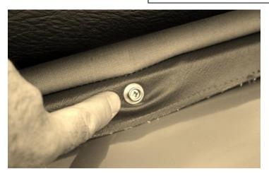
You should find that your existing hood fixes at the rear of the body using three screws with cupwashers, two in line roughly with the boot hinges and one centred between these. They screw into the timber cockpit rail. It will be necessary to fit three of the D. dot studs in these positions as shown here, replacing the cupwashers.
