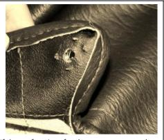
If the perforations for the prongs were made properly, piercing the facing vinyl and the reinforcing backing shown here, the top should locate easily. The plate can now be fitted.
