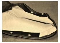
With the two sockets and two studs fitted correctly, each pocket should look like this. As an aid to fitting you will observe the correct positions are reinforced with hooding grade material.
