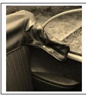
You should find that the hood attaches and fits well for the most part, held in place by the three D. dot studs and the two Lift a dot fasteners. It is now necessary to finish the job by fixing two studs and sockets to either side of the front Hood frame covering pockets, which as shown here tidies up the interior considerably.
