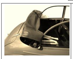
Fold the hood down neatly, remove the Lift a dot fixings on both sides, tucking them inside and out of the way.
