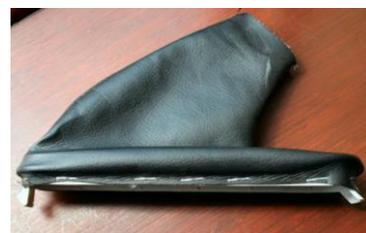
Twist handgrip to break seal -- Push rearwards & upwards to release front clip
