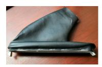
Twist handgrip to break seal -- Push rearwards & upwards to release front clip
