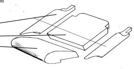
The foams are built into the base cover in the following way.
