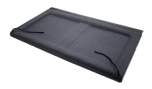
The two rubber straps at the rear of the shelf attach to clips located in the roof area above the rear lift up tailgate.
