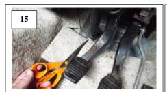
All Cars - Slit centrally to edge of column then cut a hole. Push felt behind the pedal area & trim as required.
