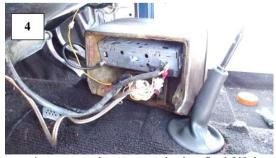
Remove securing screws on the centre console where fitted. Lift the console sideways to expose the wiring for the clock & radio. Mark all wires with tape then disconnect & remove console from the vehicle.
