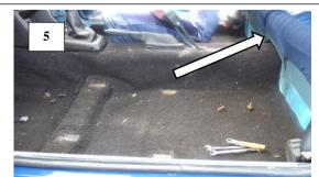
Remove centre securing screw at the bottom of the rear seat base – allowing the rear base to lift out of the way.
