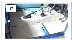
All Cars - Lay the rear floor felts in place. No overlap with tunnel felt – lightly glue in place.
