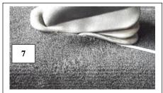
Pull the bottom edge of the hand brake gaiter through the carpet hole.
