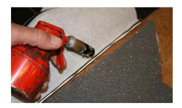
The next stage is to apply the foam padding that go over the sidebars on the seat frame. The picture here on the left shows the position of the foam in relationship to the seat cover. Apply adhesive to the side of the foam and to the stitched edge of the cover. Allow to dry slightly the push the two together. Suggest you leave them to dry properly for at least 3 hours.
