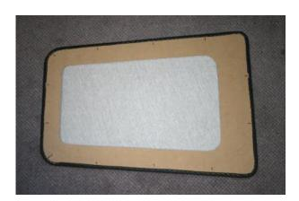
We found when we tried to remove the old backboard that the screws were rusted in place, so our new board has holes already drilled in place to miss the existing screws.
