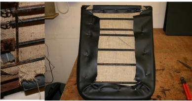
Note how the bottom of main face with the Hessian is pulled through the base frame tube. These are the pulled upwards and glued and hog ringed
