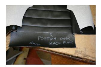
We have marked a line on the rear of the base cover to indicate that this line should be positioned on top of the rear tube. This will then make sure that the cover will fit both front and back.
