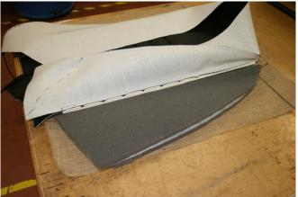
Start turning over the side skirts evenly over the foam side cushions. Pull on the piping and attach with hog rings to the base spring frame. You can then hog ring the skirt to the vertical metal wire frame as shown. At the top of each corner use seat clips to pull in the extra material to allow the backboard to sit properly.
