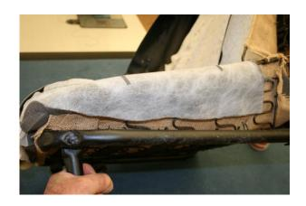
You will no doubt remember when you took your old seat covers off, that the side panels were supported by foam pads that were folded over the wire frames on the sides of the seat frame. Now that the foam pads are glued to the seat cover you will be able to fold the pad over the wire frame and glue it together to create this padding.
