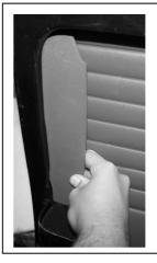
5: when the panel is lined up in the frame, allow the flaps to spring out. Make sure that the bottom of the fillet sits level on the top of the door bin.
