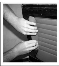
6: The last step as regards fitting the fillet is to push the back edge round until it has no more room to move. MK1 and MK2 door trim relies on tension alone to fit and retain its shape so it is important that the fillets are given a lot of pressure here. When they are finally pushed in it should be very difficult to move them at all.
