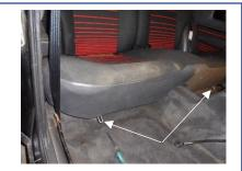
Remove the rear seat base by undoing the 2 screws either side.
