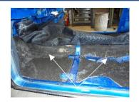
Make sure the location is correct across the cross member again and if all Is correct glue down the side of the tunnel and stick down.
