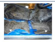
Next glue down the footwell sections all the way down the car to the outer seat mount and then stick down.
