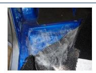
Glue the rear area of the carpet and stick down. The lip on the rear section should also be glued.
