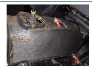
The tunnel section will be the last piece of underfelt remaining and should pull straight out with nothing else needing to be done.
