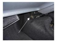
Start by laying the carpet in the car and feeding the front of the carpet under the heater matrix, Make sure the carpet sits nicely over the cross member and seat mounts.
