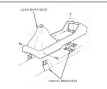
Refit the center console and all relevant screws.
