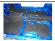
Pieces number 5 – the rear floor well sections, can be laid into place on the floor well and glued in. Minimal trimming if any is needed.
