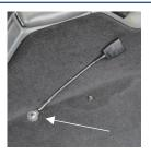
Then locate the seat belt holes in the tunnel, again make a hole in the carpet big enough to fit the bolt through. The seat belts can now be screwed into place.
