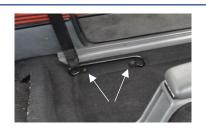
Locate the seat belt holes in the sill and make a hole in the carpet big enough to fit the bolt and screw through. The seat belt mounts can now be refitted.
