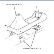
Remove the two screws by the gear lever.
