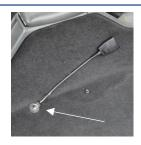
Then remove the bolt from your seat belt mount on either side of the tunnel.
