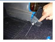
At this point the 100mm tab can be fed behind the scuttle panel.
