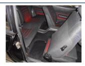
The first part of the removal process is to remove your seats. Firstly move your seat forward and remove the two 10mm bolts then move the seat back and remove the front two bolts, the seat can now be taken out of the car.
