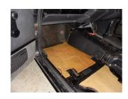
Now the carpet has been fully removed we can focus on removing the underfelt. Remove all of the pieces on the floor first.
