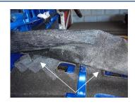
Once you are happy with how the carpet is sitting lift the driver's side and spray glue onto the top of the tunnel and stick down.
