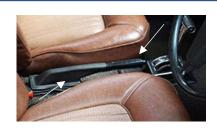
Remove the handbrake cover and grip if there is one.
