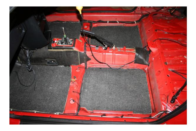
This is a fairly straightforward task; begin by laying the felt kit pieces into the foot-well areas front and rear. These will need trimming to fit exactly, in particular to clear the wiring loom and also to provide the best fit around the tunnel shape. When completed, use spray adhesive to fix the felts to the floor pan. If you are fitting a deluxe eight piece kit, stick the felts together using the adhesive also.
