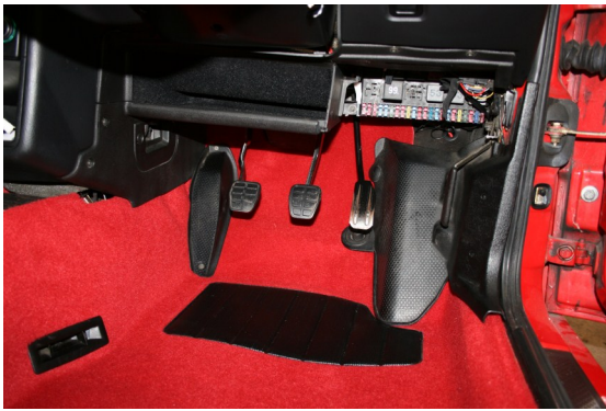
13: The front carpets overlap onto the rear, inside the foot-wells. Where the carpets meet on the sill, at this point the carpet can be trimmed back so that they finish flush against each other.
