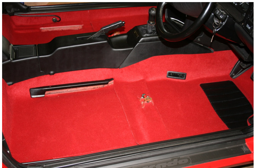
16: With the carpet re-fit complete, the rest of the interior can go back into place. When re-fitting the seats, take care if the runners are greasy not to spread this onto the new carpet or anywhere else on the interior - laying out some newspapers or old sheet to protect the interior might be a good idea. Happy Motoring!
