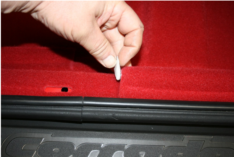
13: The front carpets overlap onto the rear, inside the foot-wells. Where the carpets meet on the sill, at this point the carpet can be trimmed back so that they finish flush against each other.
