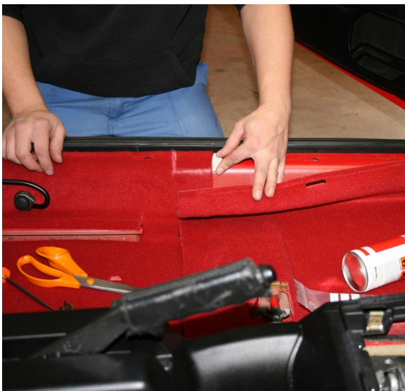
15: Make sure the holes in the sill are not obscured by carpet, and if necessary trim back with a craft knife. For LHD cars - the sill edge of the front carpets may need to be trimmed back, depending on how the wiring loom sits in the car.
