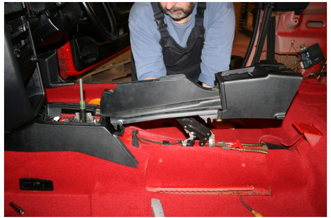
12: Re-fit the centre console sections, together with the rear seat and arm rest.
