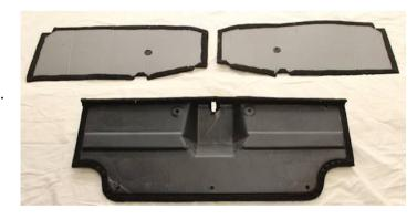
Pierce through the new carpet covering at the seven clip holes. Re fit the panel using the new clips supplied (if the old ones are unsuitable). The rear light panels are complete & just push fit into place. The creases in the boards allow them to be shaped to fit snugly in place. Your covering kit fitting is now complete.
