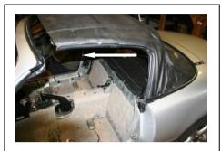
RAISE THE CONVERTIBLE TOP IN ORDER TO HAVE ACCESS TO ALL THE FIXING CLIPS AROUND THE REAR CARPET.
