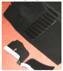
Test fit the scuttle pieces to make sure they are in the correct position. The vinyl that is sewn to the outer edge will bend around the door aperture and eventually be held in place by the draught excluder.
