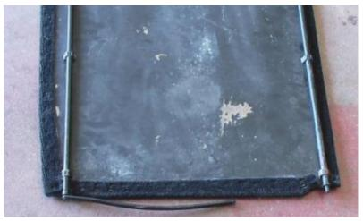
Lift out the shelf from the car and remove any staples or tacks that hold the carpet to the underside of the tray. It may be necessary to use sandpaper to clean off any old glue particles that are left on the board once the carpet is removed. Once the carpet is removed you will see how the two metal bars are held in place. Perhaps using a pair of pliers, turn back the metal flaps that go through the board. At this time you can
