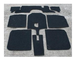
We would suggest that you start by fitting the main bulkhead felt. You may need to cut/slit the felt to allow it to sit comfortably on the bulkhead. The other two pieces lie alongside the main piece. We suggest you glue these pieces in place with an aerosol adhesive.
