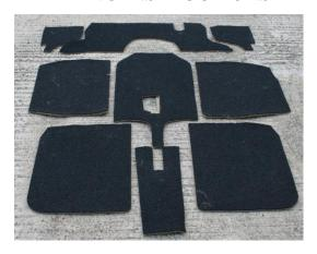
We would suggest that you start by fitting the main bulkhead felt. You may need to cut/slit the felt to allow it to sit comfortably on the bulkhead. The other two pieces lie alongside the main piece. We suggest you glue these pieces in place with an aerosol adhesive.
