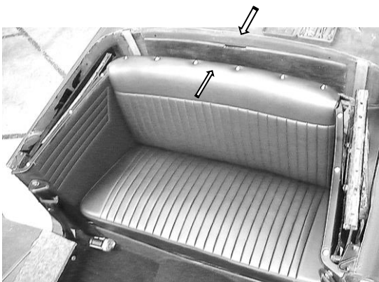
STUDS ABOVE REAR QUARTER PANELS & ALONG TOP OF REAR SQUAB ASSEMBLY.
