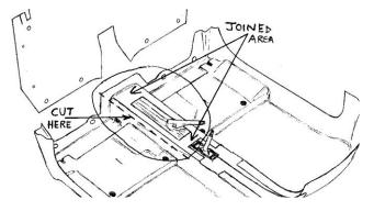
The front under felt pieces have a wedge of extra foam attached to them; this helps fill the space under the sill panels. Lay the remaining pieces in place then you can insert the new moulded sides into the car.
