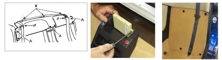
**Removal of rear Bulkhead carpet** – This carpet is held in place by eight plastic clip screws plus four push in clips. Lever out the four push in clips, which are located at the outside edges of the carpet. Use a flat-ended screwdriver to unscrew the other larger clips. Release the door draught excluder as well, as this holds the outer edges of the carpet in place.
