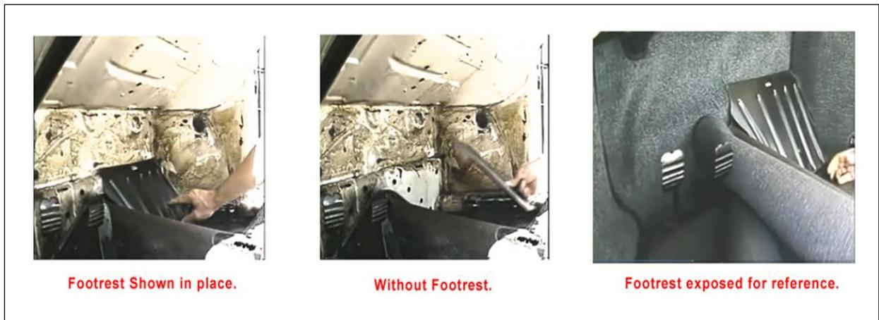
Some cars had a metal plate fitted in the passenger foot well which affects the length of the foot well carpet we need to provide. As the picture indicates this plate angles the foot well, the driver tin plate would have slots cut in for the pedals. As standard these were fitted to models after 1961 for passenger tin or after 1970 for driver tin but these are easily removed or added so best to check before ordering.
