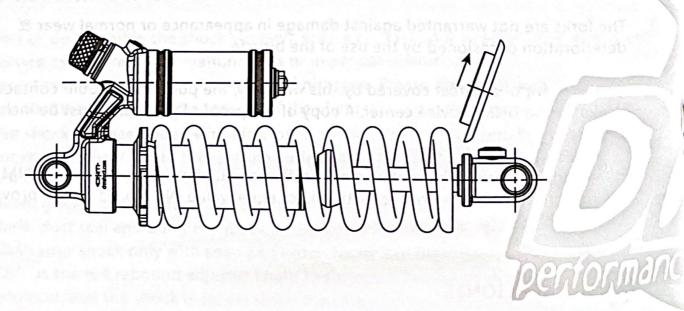
4. Install or replace the spring, and do basic maintenance and cleaning to the shock.
