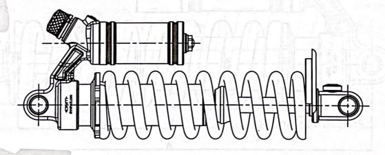
6. Tighten the Preload knob until safety ring and spring are tight and in place
