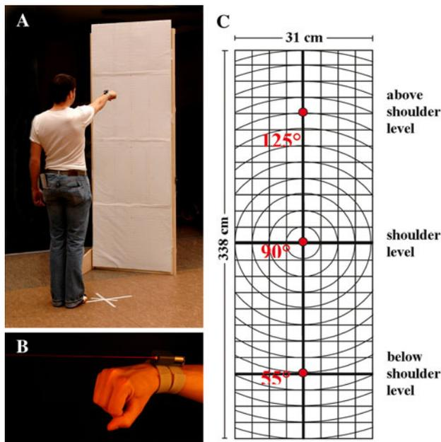
**Fig. 1** LP-ART test setup. **a** patient positioning, **b** laser pointer affixed to the dorsal aspect of the subject's wrist. **c** Target board with standardized coordinate system indicating the different angles of motion
