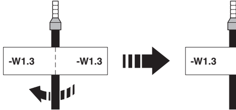
Figure 4-7 Example of a cable flag
