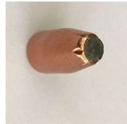
A typical jacketed bullet Note the exposed lead point
