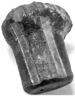
A recovered hard-cast bullet with the chemical coating stripped off in the barrel
