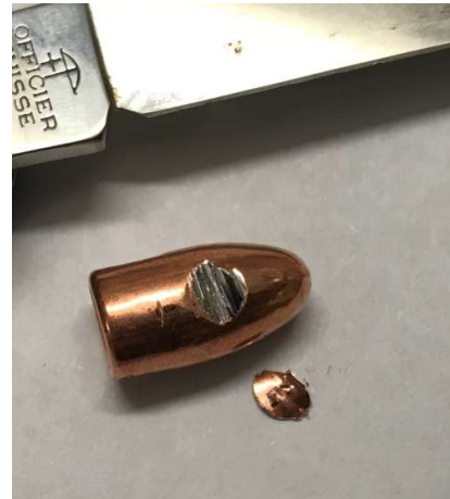
Tigershark Bullet that has passed the scrape test
