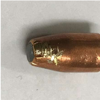
A jacketed bullet that has failed the scrape test
