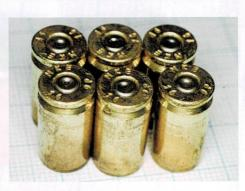
Although working near the upper recommended loads for the 9mm rounds, there was no sign of excessive pressure.
