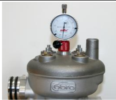
Figure 40 , Using a dial indicator to measure piston height for setting ignition timing.
