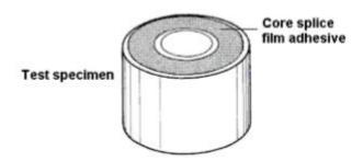
Outer and inner tubes: 12.5 mm height, aluminum alloy 5052-0 bare.
