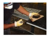
2<sup>nd</sup> Step - Apply Smooth-on to repair area.
