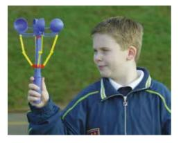
**£22.99** Anemometer Handheld or permanently fixed. A plastic Anemometer which measures wind speed in m/sec or Beaufort Scale, directly read from scale on main shaft. As the wind blows harder, the arms move further out, lifting the reading bar. Ideal for primary and lower secondary pupils.
