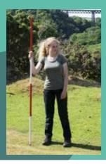
Traditional red and white 2 metre steel poles which are 27mm in diameter with a solid PVC plastic covering. They have solid steel points for easy insertion and longevity and come complete with a plastic cap. These longlife ranging poles are graduated red and white every 500mm.
