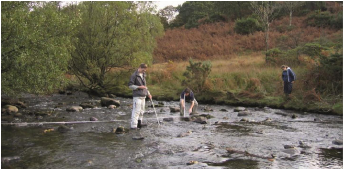
Figure 7 Measuring “Distance Out” using tape secured at each end
